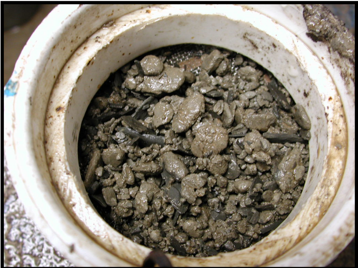
Figure 4 Cuttings from PDC bit run – Southeast Louisiana well, Iberia Parish
