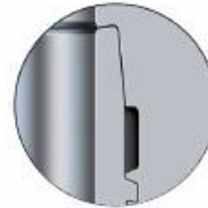
Internal torque shoulder, metal-to-metal seal and lubricant relief groove
