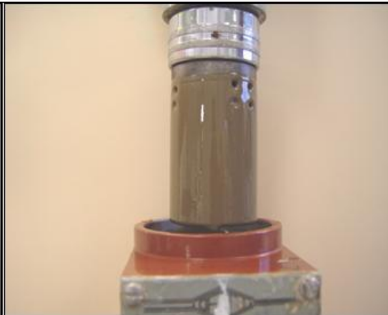
Sleeve Coated with 13.2 ppg SBM
