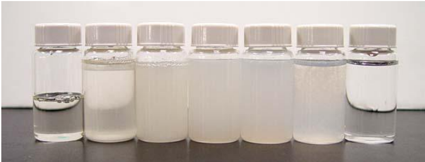
14.8 lb/gal Zn-CaBr 2 with synthetic formation water.
