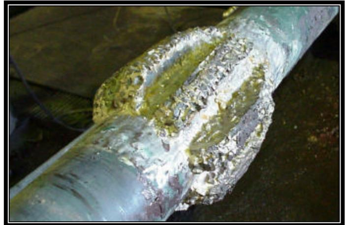
Figure 13 - Follow Mill still in gauge after 8 hours.
