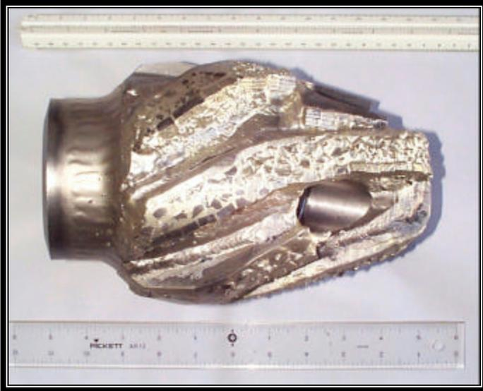
Figure 3 - State of the art dressing of preformed and crushed tungsten carbide on Lead Mill of One-Trip Sidetracking System mill.
