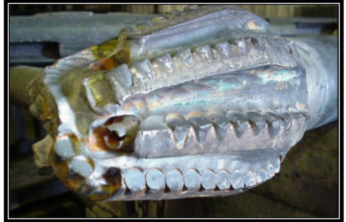
Figure 12 - ETC Lead Mill after 8-hour sidetrack.
