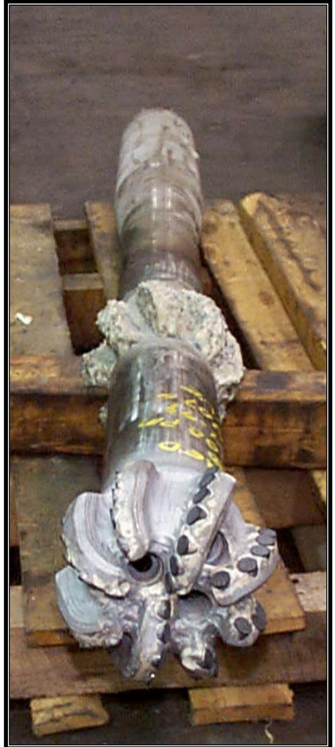
Figure 2 - Standard PDC Bimill for 7-in. casing with only PDC cutting structure on Lead Mill profile and preformed and crushed tungsten carbide dressing on the Follow Mill profile.
