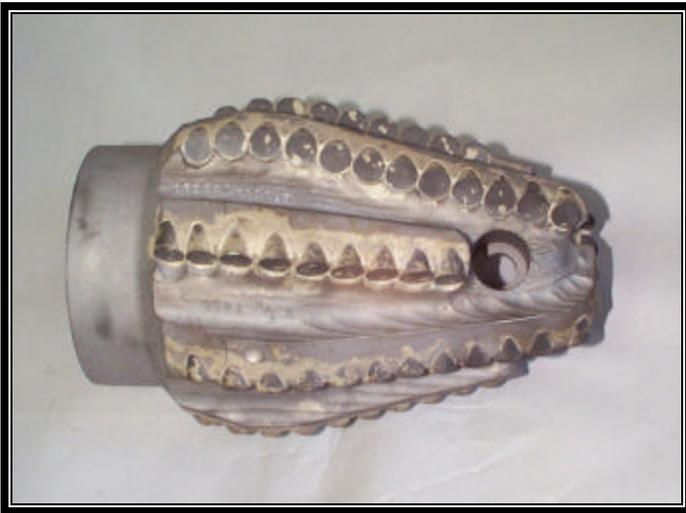
Figure 11 - Lead Mill dressed with ETC cutters. Hole through the mill is used for attaching it to whipstock.
