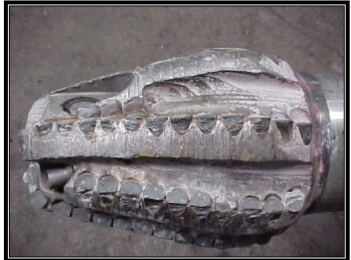
Figure 14 - Lead Mill with ETC cutting structures after milling 8-ft. of casing window and drilling 10-ft. of sandstone-shale formation in 2.25 hrs.
