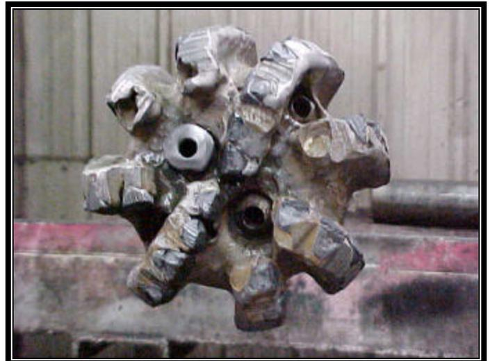
Figure 6 - PDC Lead Mill is 1/16-in. under gauge after cutting a window through 7-in. N-80 casing and drilling 565-ft. lateral in 16.3 hours and in one run.
