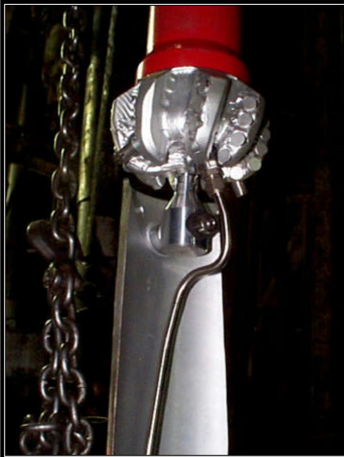
Figure 4 - First method for attaching PDC Bimill to hydraulic whipstock assembly.
