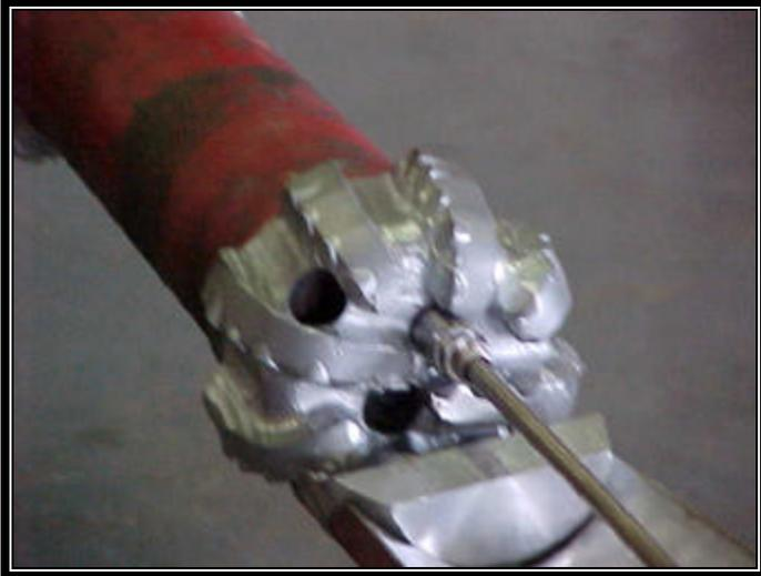
Figure 10 - New connector between whipstock and PDC Bimill used on West Texas and San Juan Basin.
