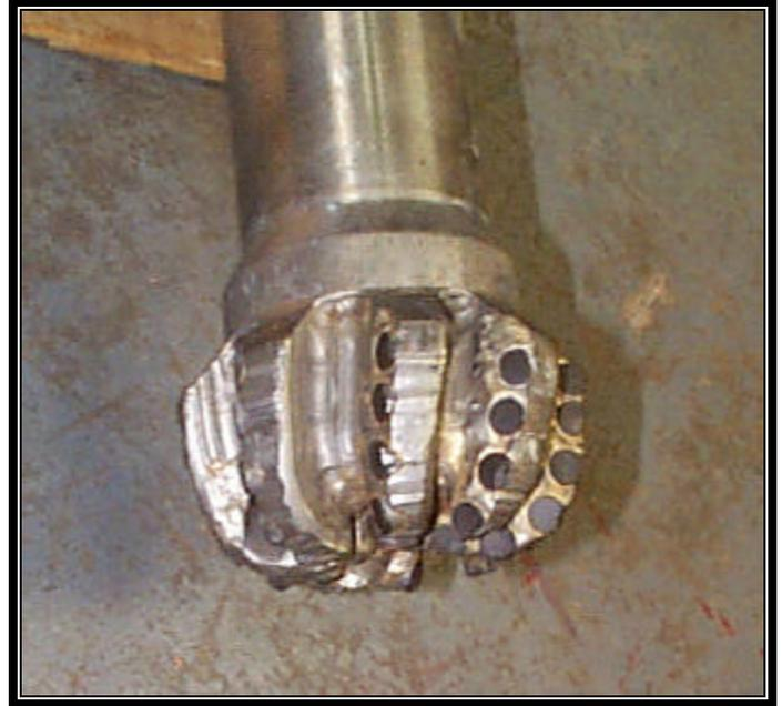
Figure 5 - PDC Lead Mill only 1/8 in. under gauge after milling a window through 7-in. casing and drilling 560 ft. lateral in 12 hours and in one run.
