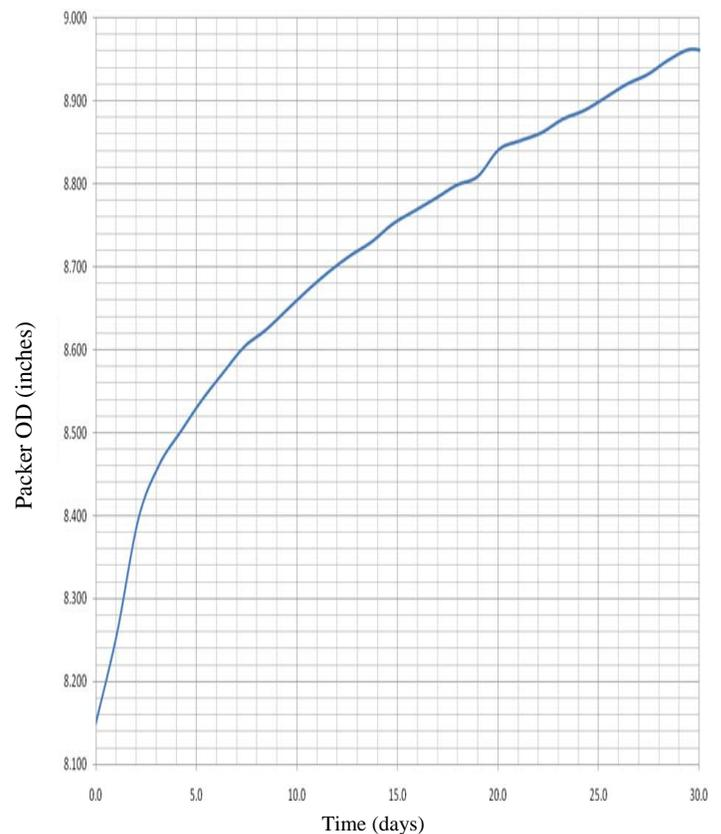
**Fig. 4** Elastomer swell test profile.
