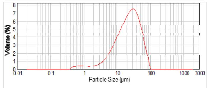
**Fig. 3** Particle size analysis of the reservoir drilling fluid.
