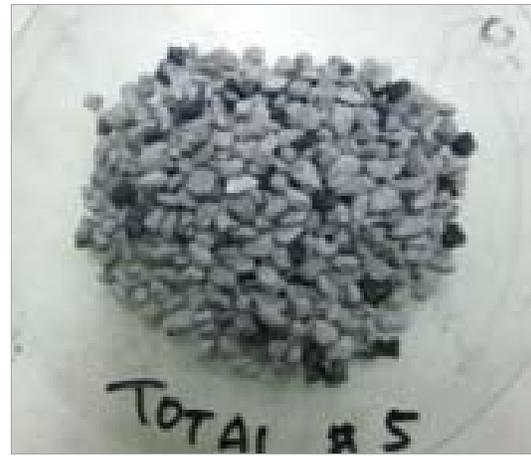
**Fig. 2** Shale erosion sample post-test.
