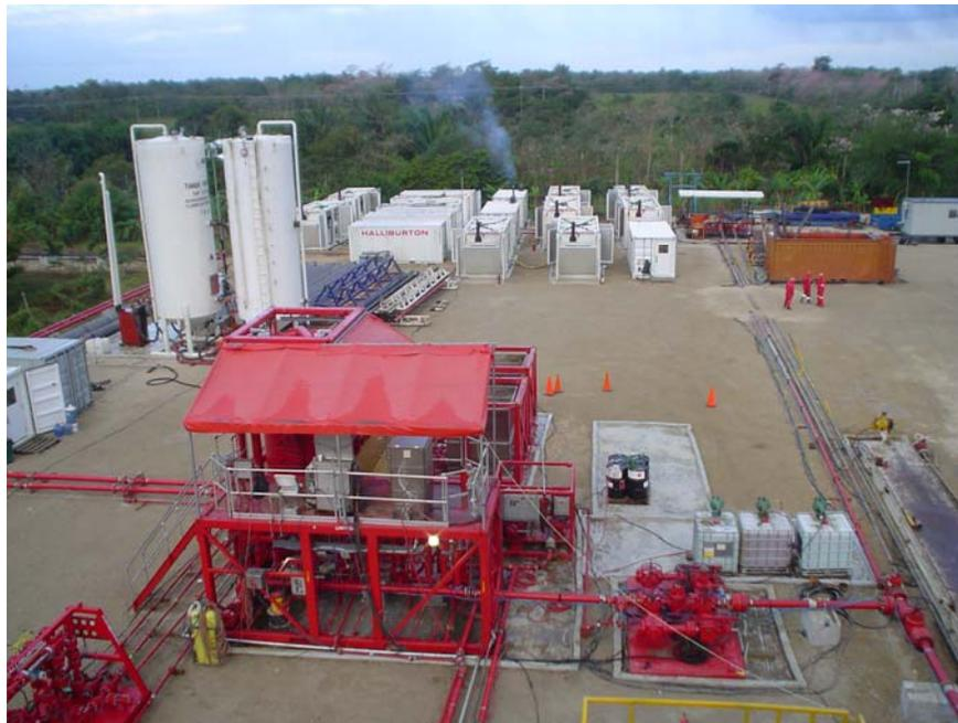
**Figure 3 —Equipment rigged up at location for MPD onshore field case.**
