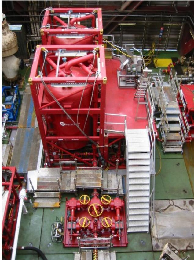
**Fig. 2 - Equipment rigged up for MPD offshore field case.**
