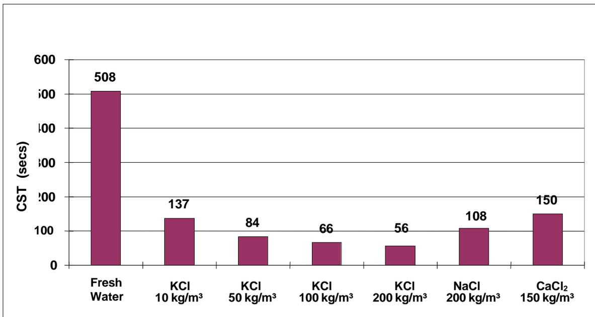
**Figure 3. Effect of various inhibitive drilling fluids on erosion and swelling of the Dogger shale**
