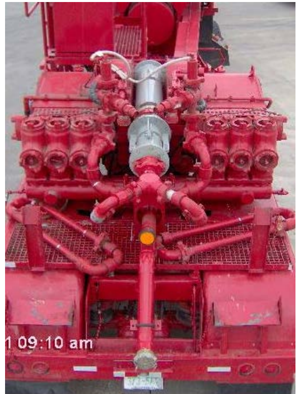
Figure 8 - Pumps are fed from rear of the trailer - all high pressure lines remain on the pump unit.
