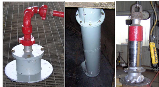
Figure 4 Prototype 1 general arrangement of 8½ “ PDC bit and sub set into 10 inch casing in a mixing pit –
