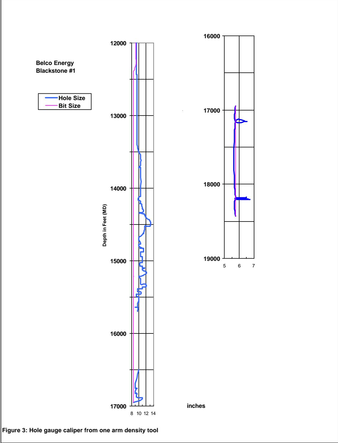
Figure 3: Hole gauge caliper from one arm density tool
