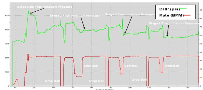
Figure 3- shows the pump rates and pressures during a frac to illustrate the ball drops and ball landing.
