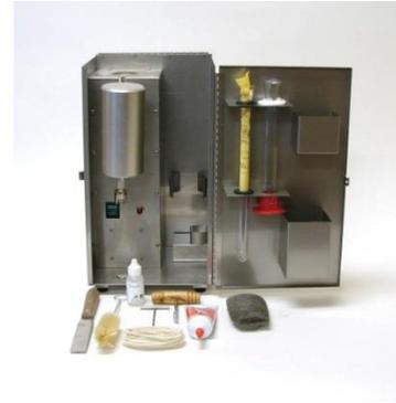
Figure 1 Retort distillation kit
