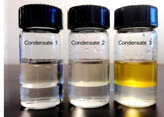
**Figure 3.** Condensate and their interface with 10% KCl brine.
