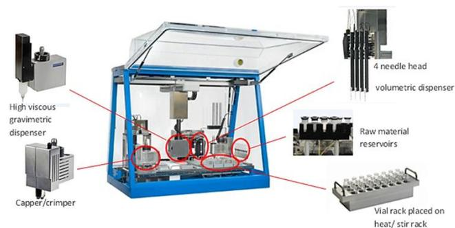
**Figure 1.** Image of “Swing Emulsifier” platform and robotic tools used for the microemulsion formulations
