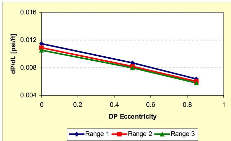
Figure 2: Pressure Loss vs drill pipe eccentricity and rheology range at 800 gal/min.
