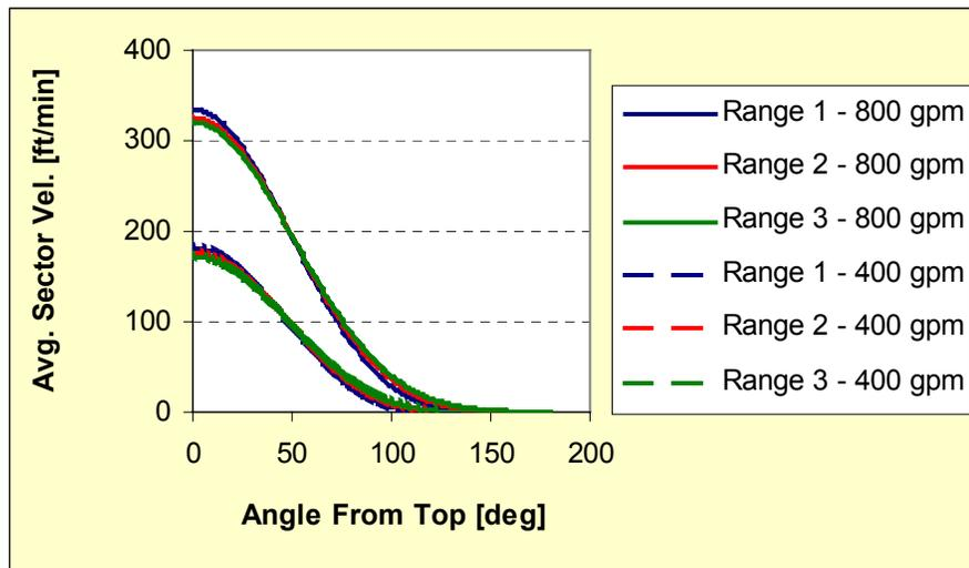
Figure 6: Average sector velocity vs angle from top of annulus, rheology range, and pump output.
