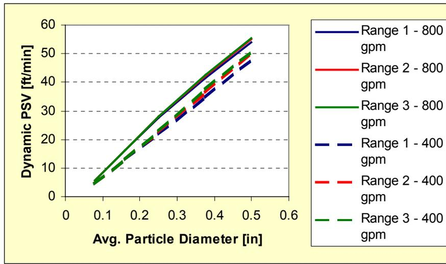
Figure 5: Dynamic PSV by particle diameter, rheology range, and pump output.
