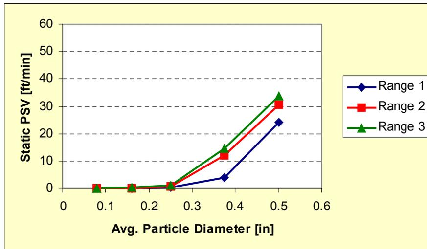
Figure 4: Static PSV by particle diameter and rheology range.
