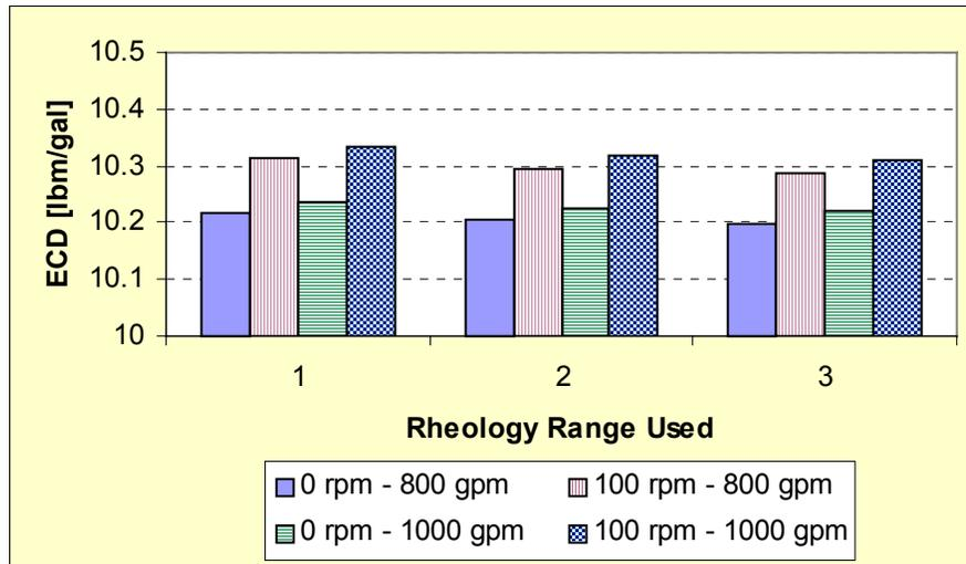
Figure 3: Calculated ECD by pump rate and drill pipe rpm.
