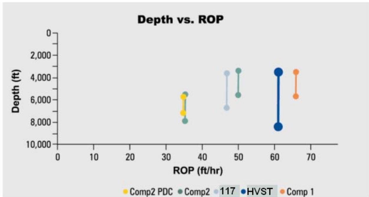
Figure 16 – 12-1/4” Bit run comparison of one HVST bit run vs several competitor tricone 117 ST bit offsets and one competitor PDC bit offset. The HVST bit more than doubled the footage of the best offset, and drilled faster than all the offsets that approached this depth range.
