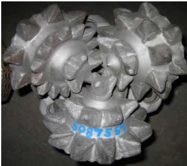
Figure 15 – 9-7/8” HVST bit run #2 which achieved 74 fph section ROP. The dull is in excellent condition after 4392’ of drilling with a dull grade was 1 1 WT A E I CT TD.
