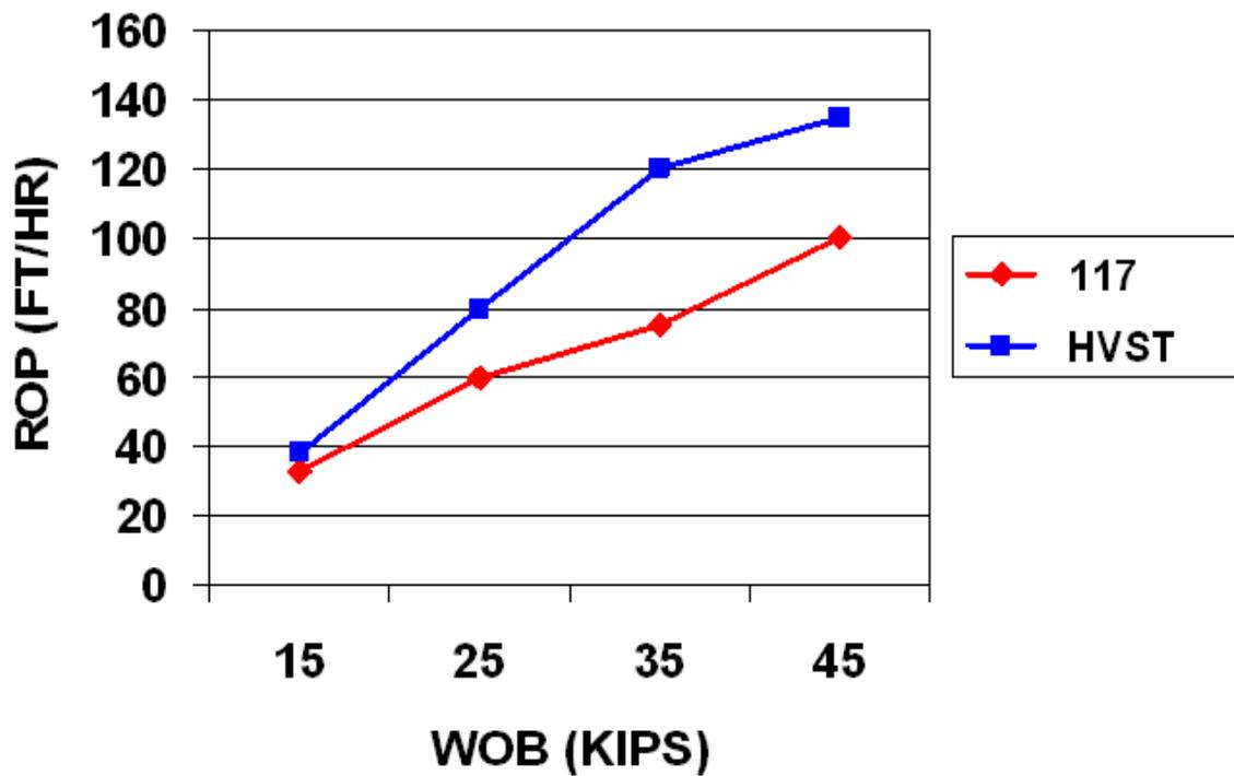
Figure 4 – Laboratory high pressure drilling simulator test results under “Fast Surface Hole” test conditions: 8-1/2” bits, 1000 psi bottomhole pressure, 9.5 ppg WBM, Catoosa shale, 120 rpm.
