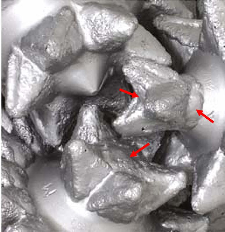
Figure 9 – Complete spearpoint coverage with hardfacing (shown by arrows).
