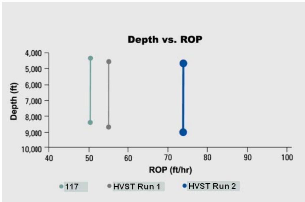
Figure 14 – 9-7/8” Bit run comparison of two HVST bit runs vs one conventional 117 ST bit offset.
