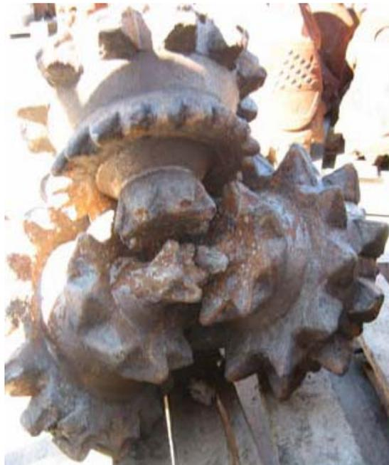
Figure 19 – 17-1/2” HVST dull in good condition after 4978’ of drilling, the dull grade was 1 2 WT G E I E R HR.
