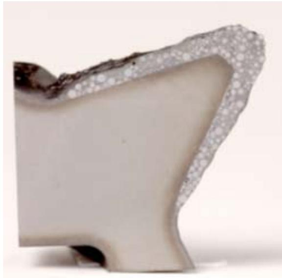
Figure 6 – Cross-section view of a Pyramid inner row tooth.
