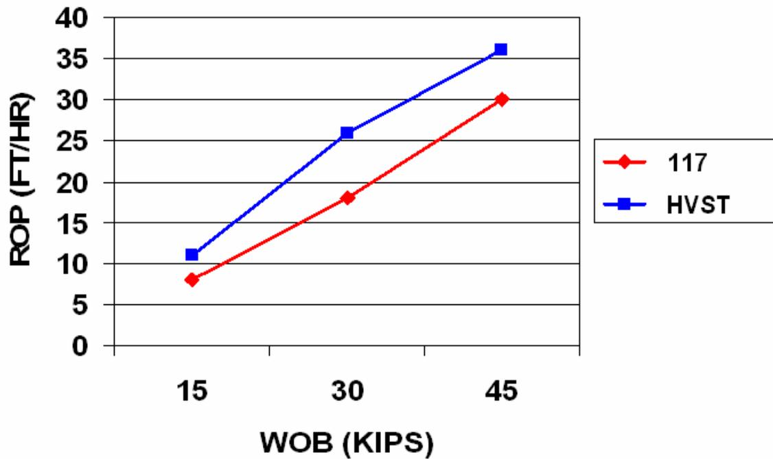
Figure 3 – Laboratory high pressure drilling simulator test results under “Deep Land” test conditions: 8-1/2” bits, 4000 psi bottomhole pressure, 9.5 ppg WBM, Mancos shale, 120 rpm.
