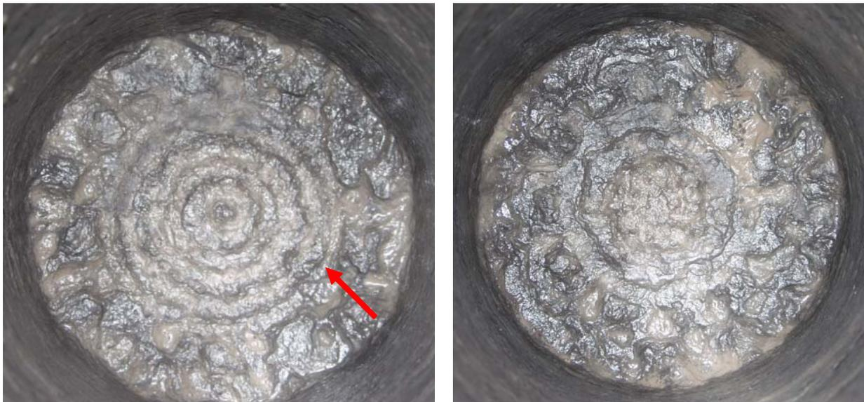
Figure 8 – Laboratory bottomhole patterns for the 9-7/8" HVST bit (left) and the standard 117 bit (right).
