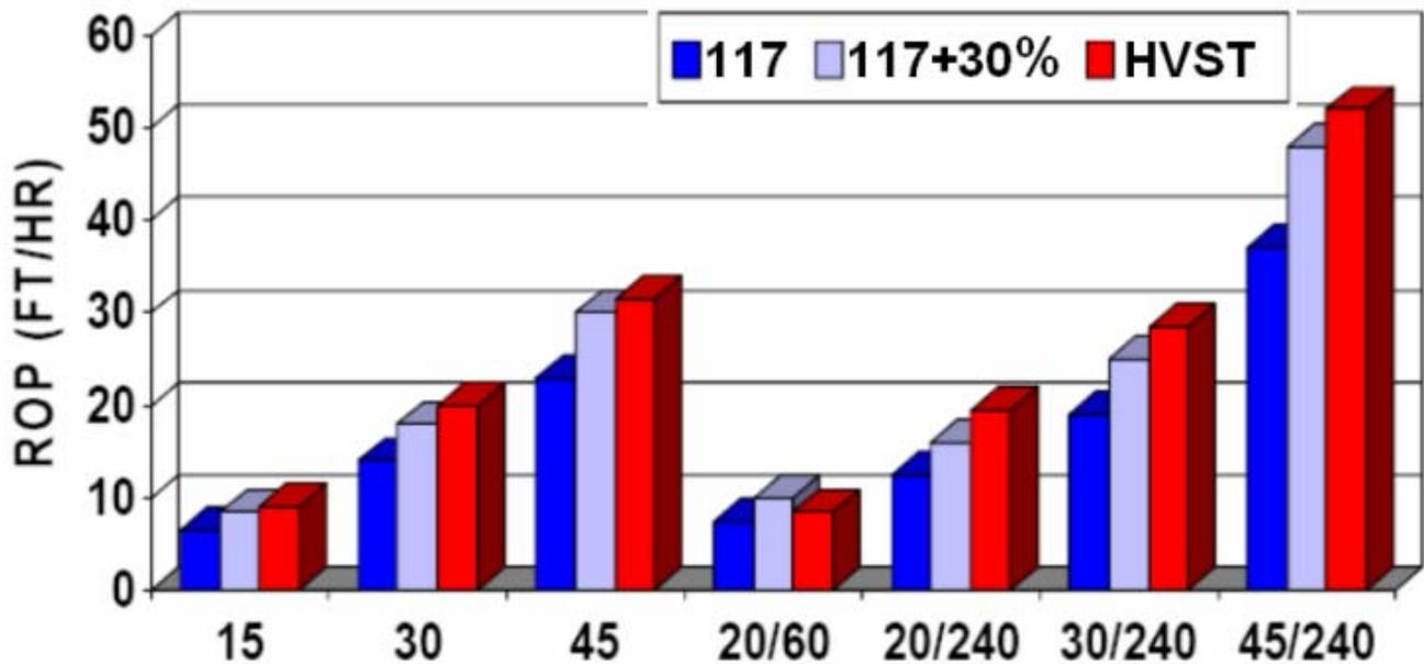
Figure 2 – Laboratory high pressure drilling simulator test results under “Heavy Mud/Deep Hole” test conditions: 8-3/4” bits, 6000 psi bottomhole pressure, 14 ppg WBM, Catoosa shale. Operating parameters: 15, 30 & 45 klbs at 120 rpm for left side of graph; WOB/RPM for 4 comparisons on right side of graph).
