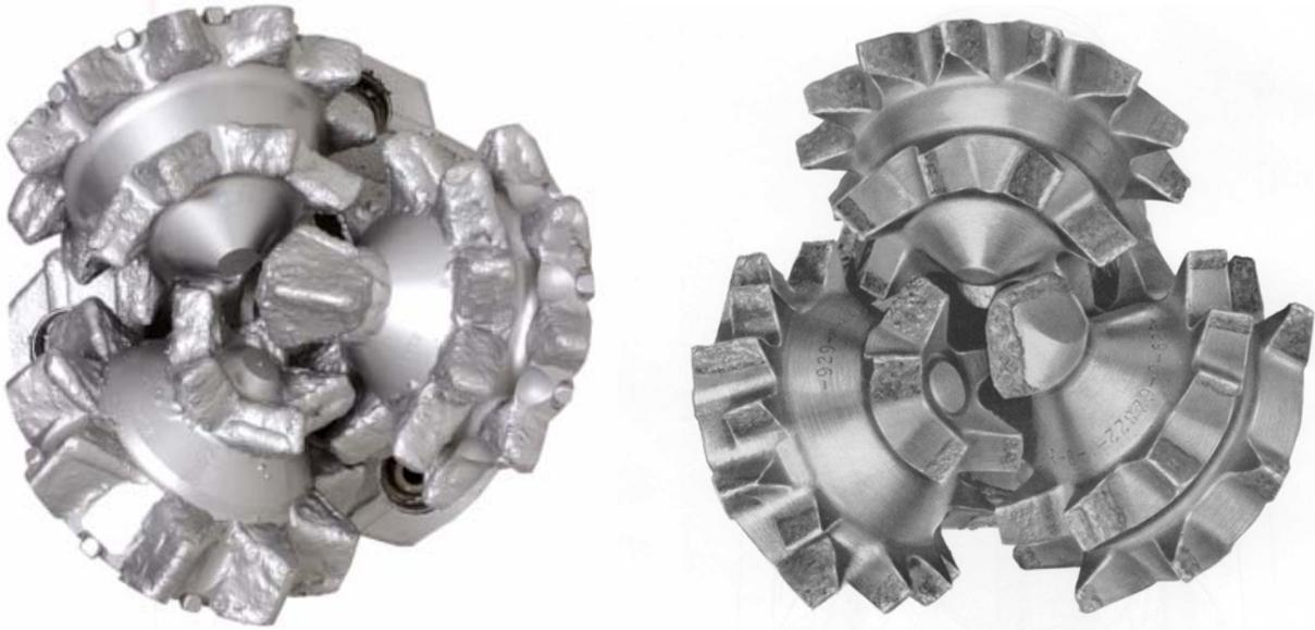
Figure 1 – Modern premium 9-7/8” IADC Class 117 ST Bit (left) vs. a 1957 era IADC Class 115 ST bit (right). Note both bits have similar row counts, tooth counts, tooth projection, cone offset, etc.
