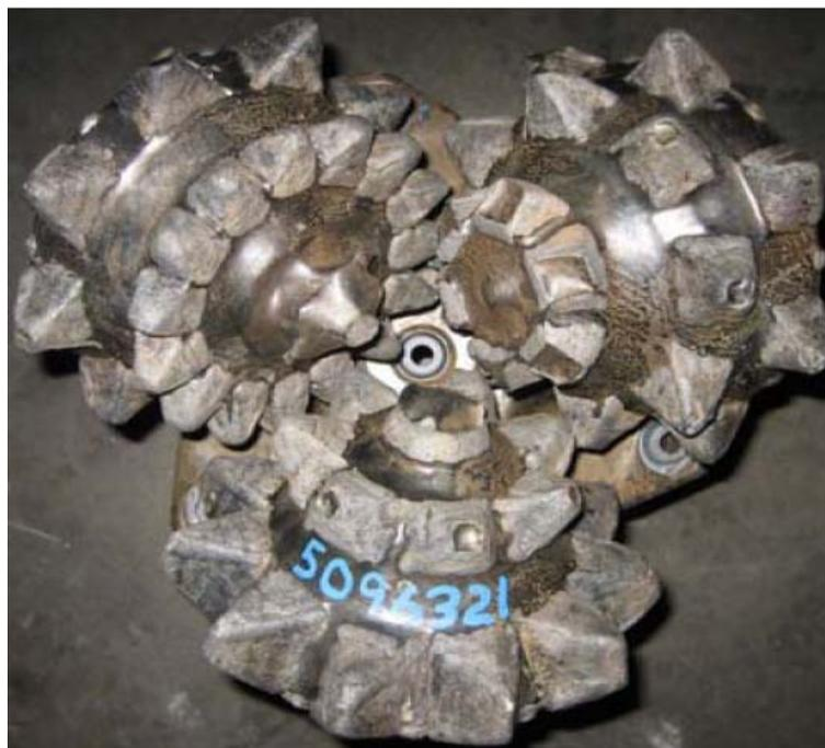
Figure 17 – 12-1/4” HVST dull in good condition after 4865’ of drilling, the dull grade was 2 1 WT A E I ER BHA. Note the nose row erosion from extended service under high flowrates and a centerjet.
