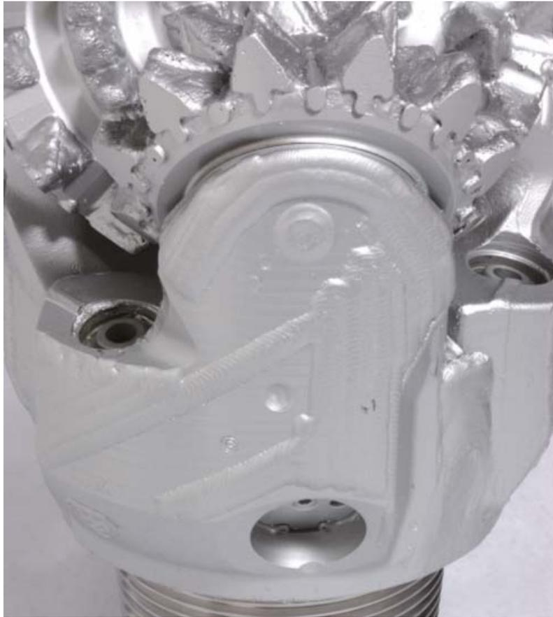
Figure 13 – Improved shirrtail and leg hardfacing on 12-1/4” HVST bit reduces the damaging effects of hole-wall contact.
