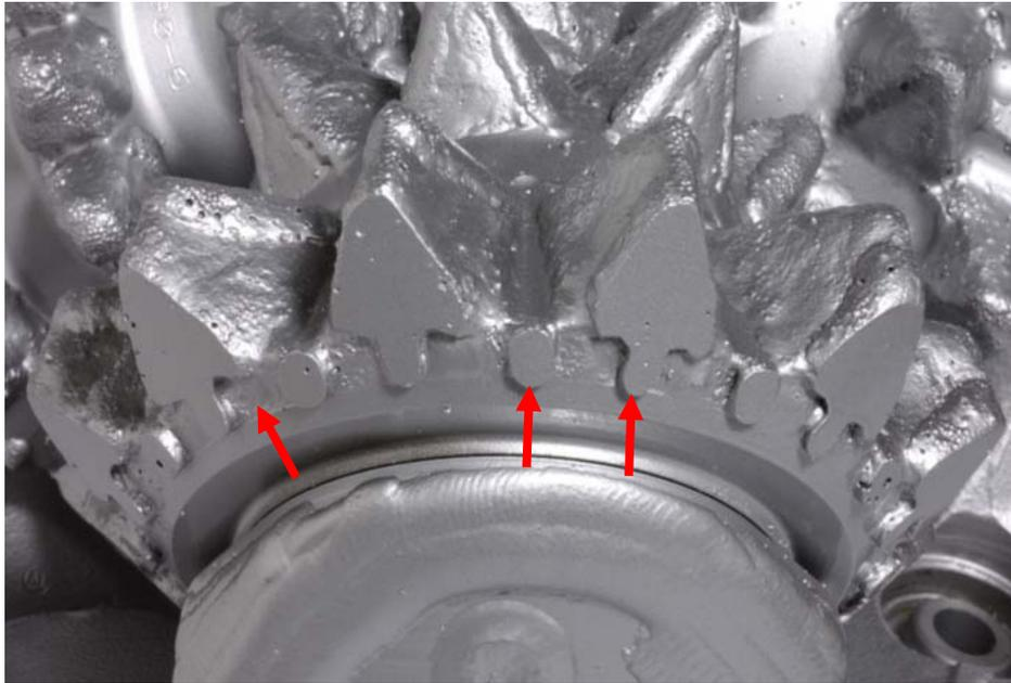
Figure 11 – Welded gauge trimmer pads, or bar trimmers, shown by two vertical arrows. Note the continuous ring of hardfacing on the cone gauge surface between the bar trimmers, shown by the inclined arrow.
