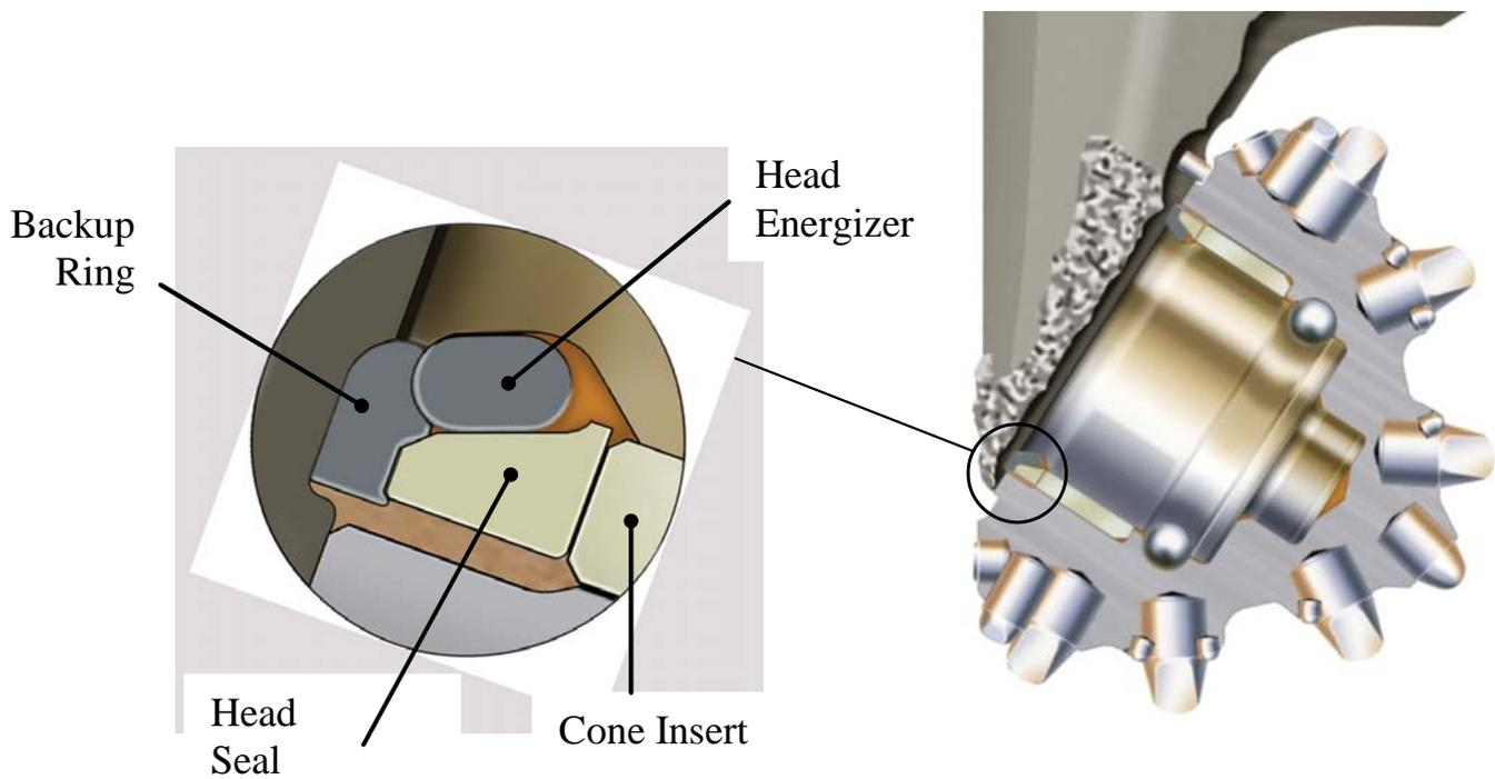
Figure 12 – Second generation single energizer metal seal bearing (SEMS2) with enlarged view of seal package (circa 2005).
