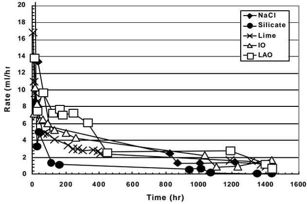
Figure 11. Rate of fluid loss over 24 hours at 1000 RPM.
