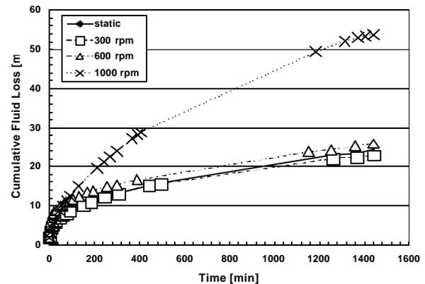
Figure 8. Effect of shear rate on the 24-hr fluid loss in a lime/salt drilling fluid.
