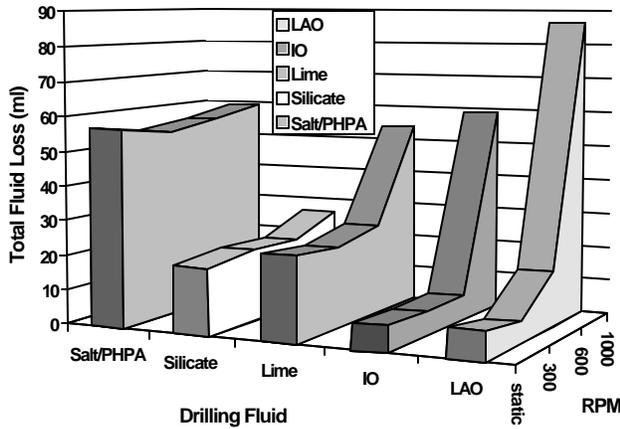
Figure 3. Summary of the cumulative fluid loss of all measured drilling fluids.
