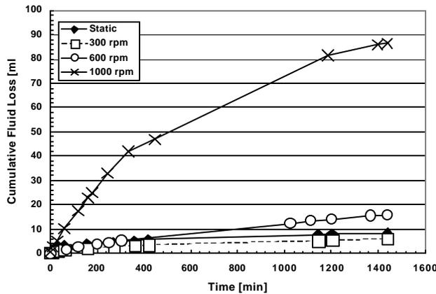
Figure 5. Effect of shear rate on the 24-hr fluid loss in a SBM with LAO as base.
