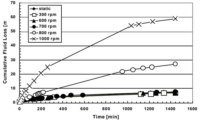
Figure 4. Effect of shear rate on the 24-hr fluid loss in a SBM with internal olefins as base.
