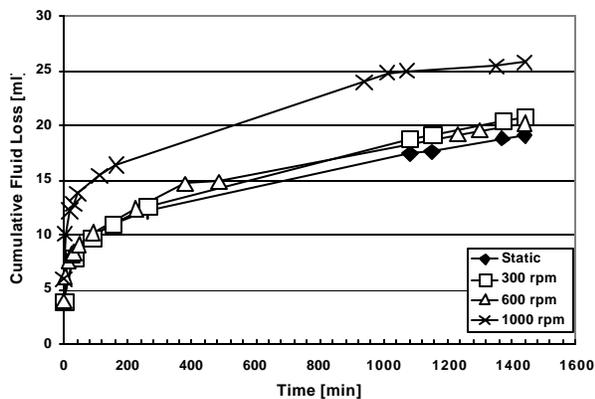
Figure 7. Effect of shear rate on the 24-hr fluid loss in a silicate drilling fluid.
