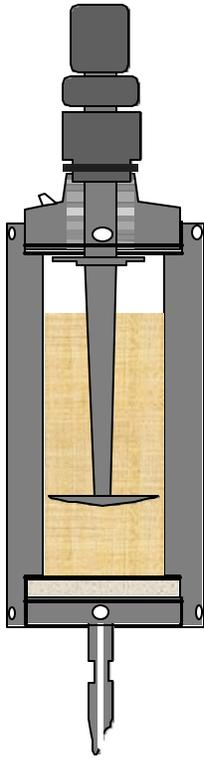
Figure 1- Schematic of dynamic fluid loss cell.
