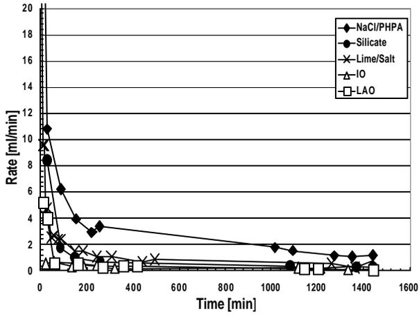
Figure 9. Rate of fluid loss over 24 hours at static conditions.
