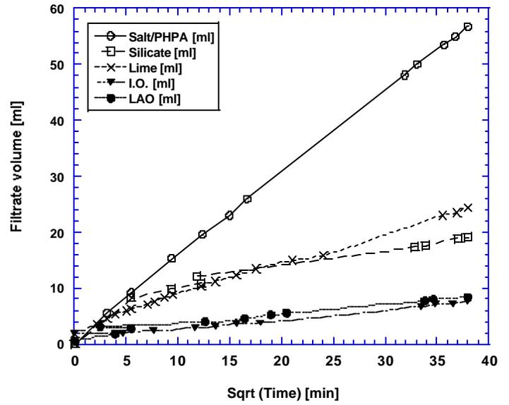
Figure 2. Static fluid loss across a 5 micron aloxite disk in 24 hours.
