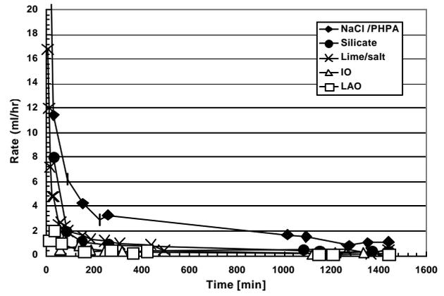
Figure 10. Rate of fluid loss over 24 hours at 300 RPM.
