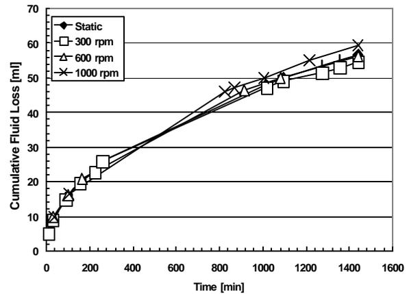
Figure 6. Effect of shear rate on the 24-hr fluid loss in a NaCl/PHPA drilling fluid.
