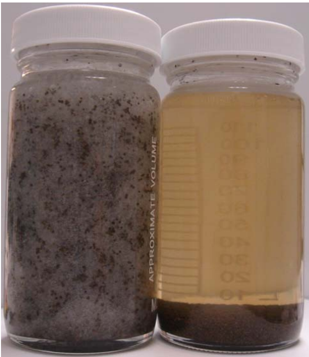
Figure 2. Photo shows ceramic particle suspension after 90 minutes. Both test bottles have 2% bv gel-forming surfactant. Test bottle on left contains 0.077% bw nanoparticles and shows strong pseudo-crosslink of thread-like micelles.
