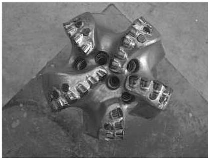
**Figure 7.** PDC bit used in the field test.
