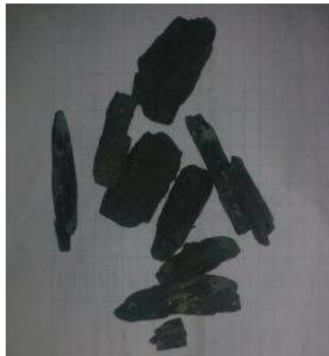
Figure 2: Long angular cuttings are observed at the shaker screen because of wellbore instability
