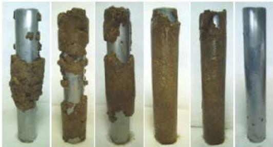
Figure 1: Accretion profile over time at 5, 10, 20, 40, 60 and 80 minutes.
