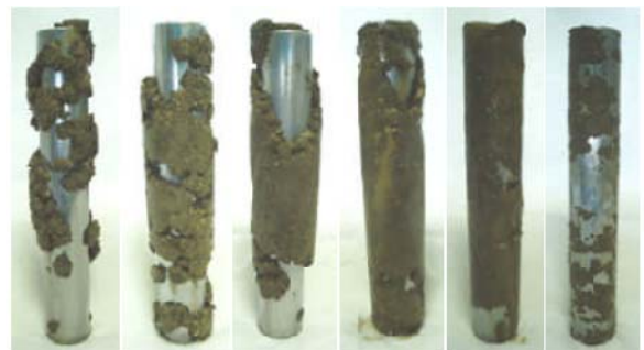
Figure 3: Oxford clay accretion profile over time ( 5, 10, 20, 40, 60 and 80 minutes).
