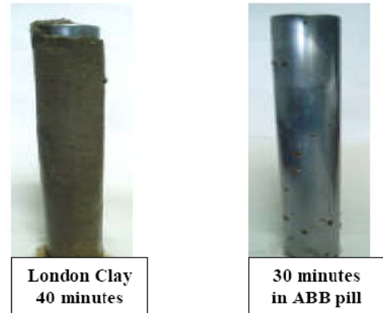
Figure 12: Effect of new anti-balling pill on accreted London clay.
