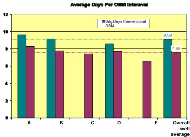
Fig. 3 – Comparison of average drilling days per interval by rig. (green is conventional invert, red is new one-drum system).
