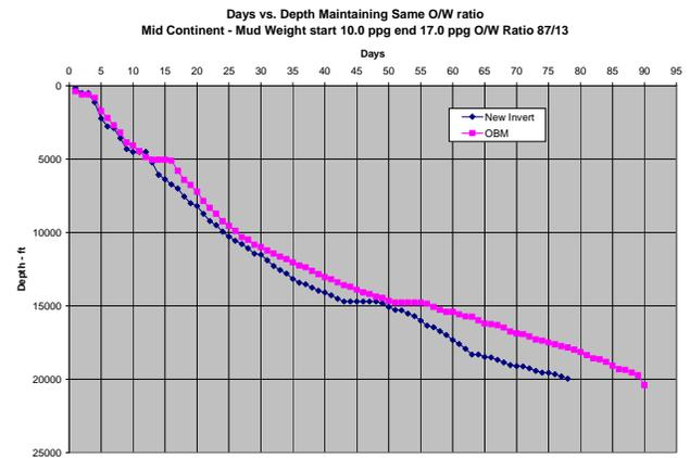
**Fig. 1 – Comparison of drilling days vs depth.**
