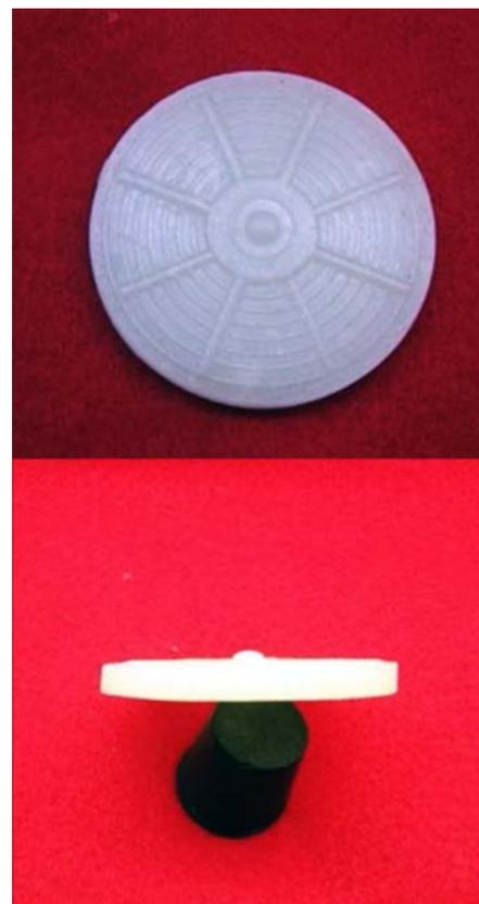
**Fig. 16—Reinforced amorphous PLA wafers after testing in HP/HT cells with a 0.25-in. hole and wrapped screen at  $180^{\circ}\text{F}$  under 500 psi for 2 hr.**
