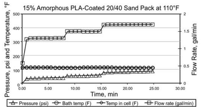
Fig. 4—Cell testing of 15% amorphous PLA coated 20/40 sand pack at 110°F.
