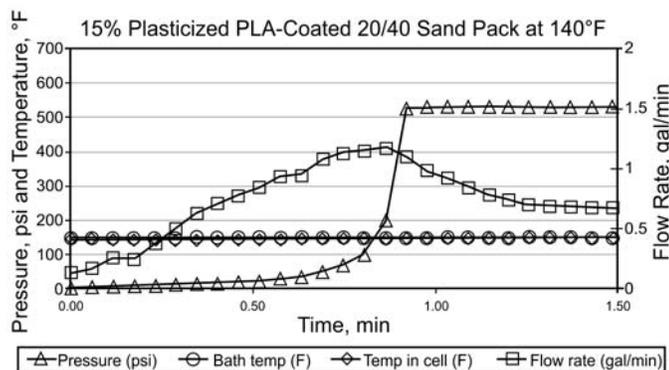
**Fig. 7—Cell testing of 15% plasticized PLA coated 20/40 sand pack at 140°F.**
