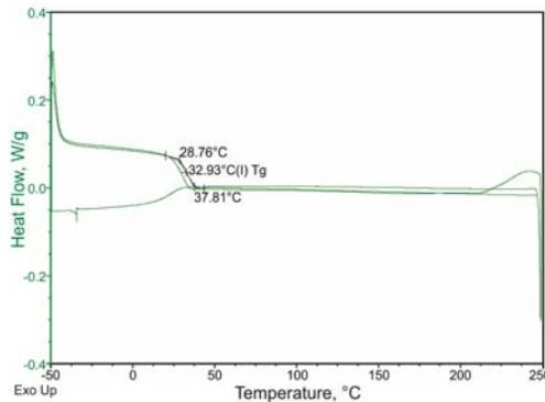
Fig. 3—DSC traces recorded for plasticized PLA (made with 15 PHR Tributyl Citrate) in a heat-cool-heat cycle. Tg was determined to be 33°C.
