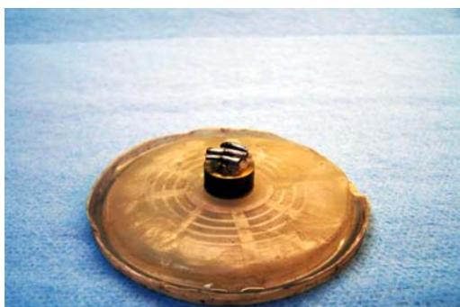
**Fig. 12—Amorphous PLA wafers after testing in HP/HT cells with a 0.25-in. hole and wrapped screen at 180°F under 200 psi.**
