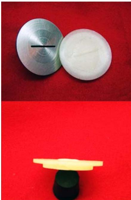
**Fig. 17—Reinforced amorphous PLA wafers after testing in HP/HT cells with a 1.5-in. length  $\times$  0.065-in. width  $\times$  0.125-in. thick slot model at 180°F under 500 psi for 2 hr.**
