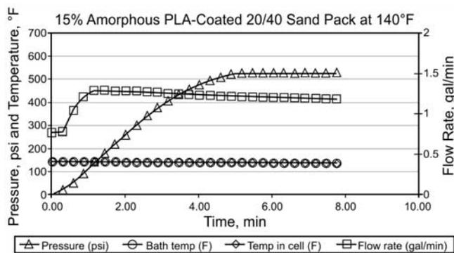
**Fig. 6—Cell testing of 15% amorphous PLA coated 20/40 sand pack at 140°F.**
