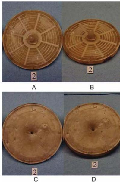
**Fig. 9—Amorphous PLA wafers after testing in HP/HT cells with a 0.25-in. hole at 180°F under 140 psi.**
