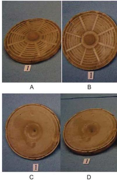
**Fig. 8—Amorphous PLA wafers after testing in HP/HT cells with a 0.44-in. hole at 180°F under 100 psi.**
