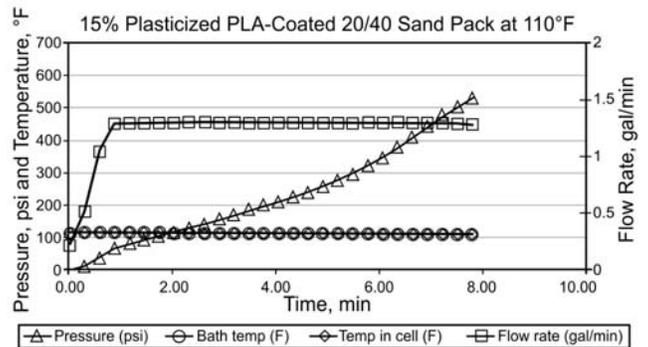
Fig. 5—Cell testing of 15% plasticized PLA coated 20/40 sand pack at 110°F.
