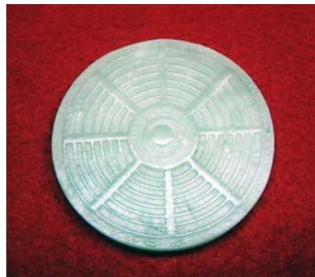
**Fig. 15—Reinforced amorphous PLA wafers after testing in HP/HT cells with a 0.25-in. hole and wrapped screen at  $180^{\circ}\text{F}$  under 200 psi for 2 hr.**
