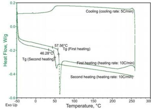
Fig. 2—DSC curves of amorphous PLA alone.
