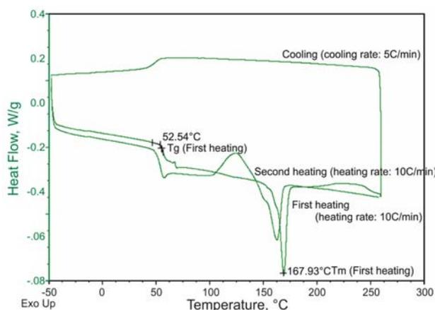
**Fig. 14—DSC curves of the composite (70% amorphous PLA, 30% crystalline PLA powder).**
