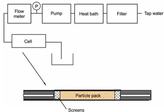
Fig. 1—Test setup and flow cell.
