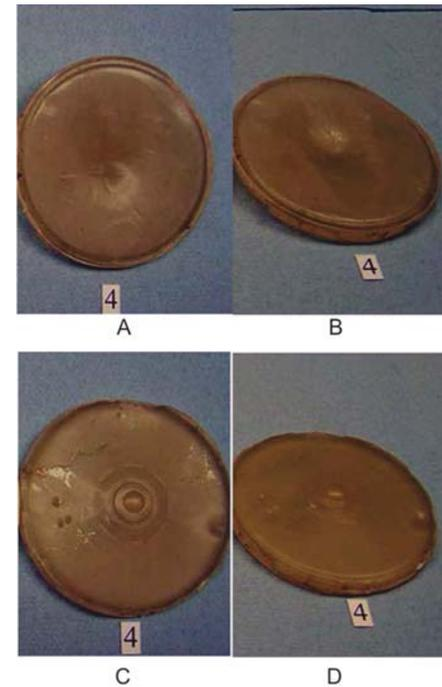
**Fig. 11—Amorphous PLA wafers after testing in HP/HT cells with a hole of 0.25-in. at 130°F under 200 psi or 2 hr.**
