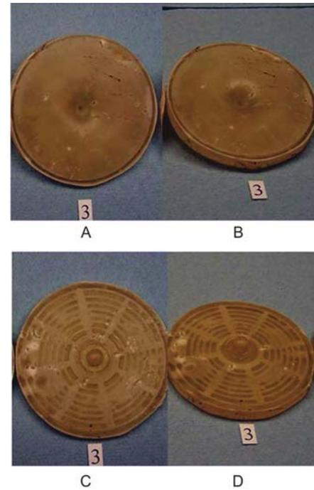
**Fig. 10—Amorphous PLA wafers after testing in HP/HT cells with a 0.25-in. hole at 150°F under 200 psi for 2 hr.**
