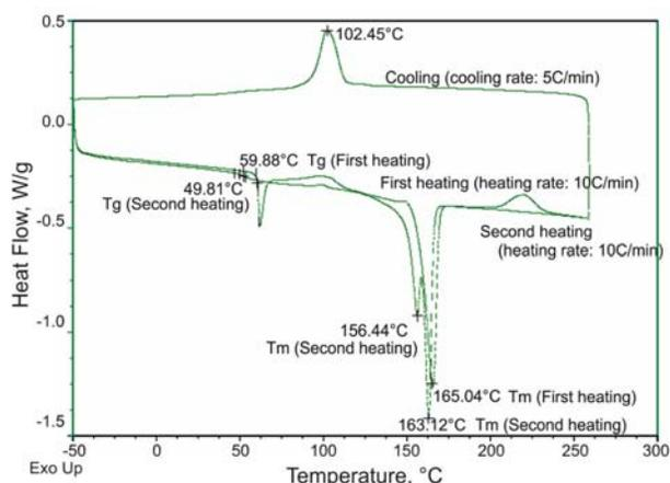
**Fig. 13—DSC curves of crystalline PLA.**
