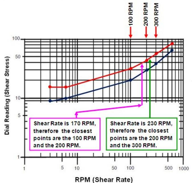
Fig. 3 – Two Rheogram Plots with 2 Closest Shear Rates
