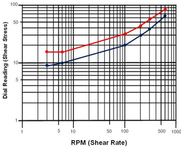
Fig. 1 – Two Rheogram Plots of Viscometer Readings
