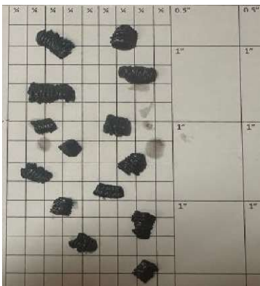
Image 2 – Example cutting sample, excellent integrity and no cavings
