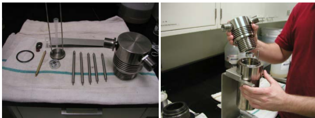
Figs. 3a-b: Full set of internal PVTP components and head installation with the large piston in place.
