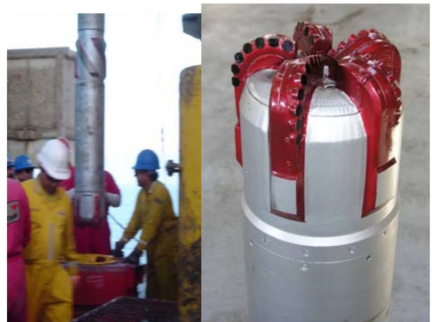
Fig. 5. 9 5/8-in. x 12 1/4-in. Displaceable CWD Bit
