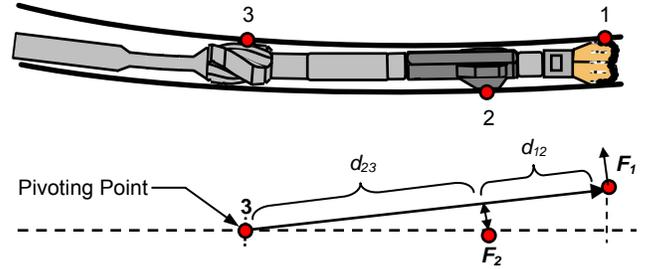
Figure 10: The pivoting point in push-the-bit mode
