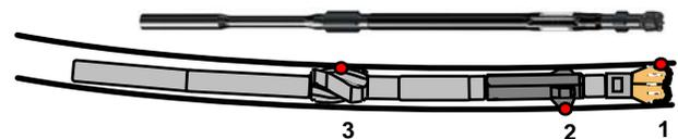
Figure 3: RSS in push-the-bit configuration
