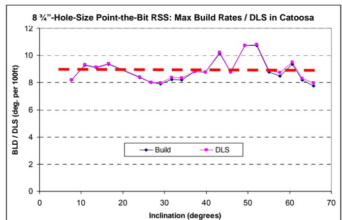
**Figure 17:** The 8 3/4”-hole-size point-the-bit RSS: Continuous Build-up Test in Catoosa.
