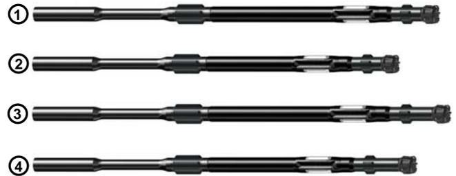
**Figure 14:** Various push-the-bit BHAs tested in RMOTC:
