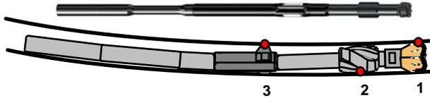
**Figure 6:** RSS in point-the-bit configuration
