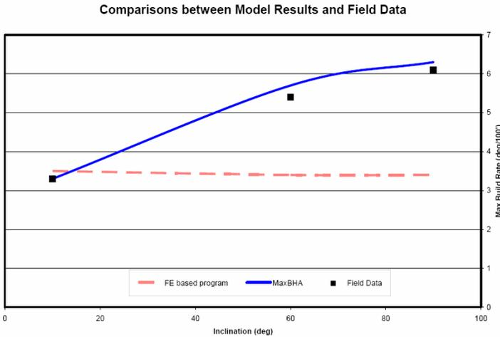
**Figure 7:** Maximum build-rate changes depending on the hole inclination with the third-party 8 1/2"-hole-size point-the-bit RSS. (Excerpted from SPE 101186)
