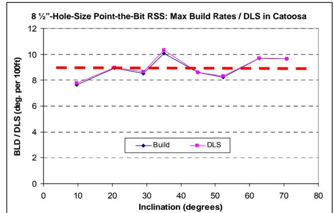
**Figure 16:** The 8 1/2”-hole-size point-the-bit RSS: Continuous Build-up Test in Catoosa.
