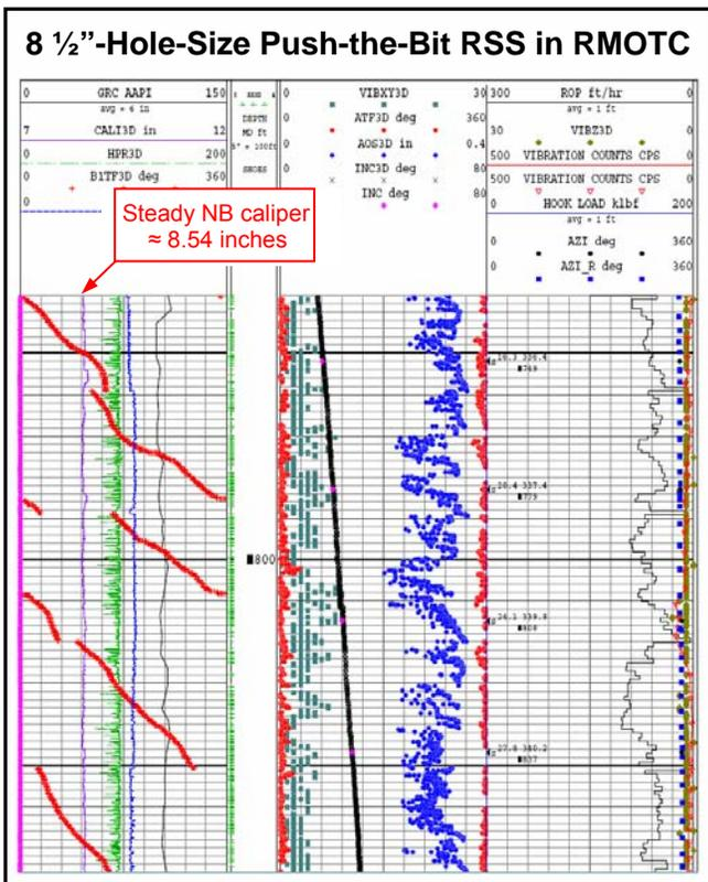
Figure 19: The maximum build rate test with an 8 1/2-inch-size prototype push-the-bit BHA (w/ 88% deflection).
