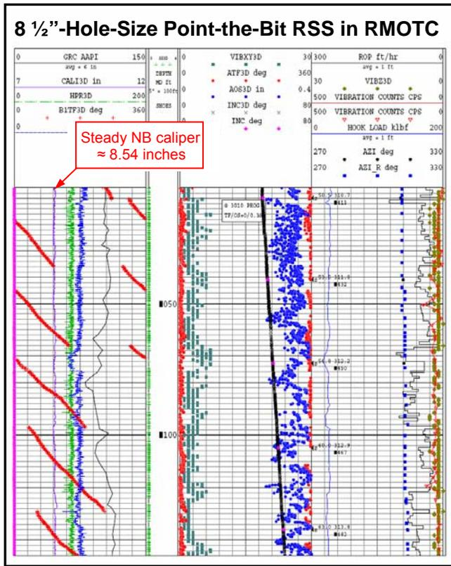
Figure 18: The maximum build rate test with an 8 1/2-inch-size commercial point-the-bit BHA (w/ 98% deflection).
