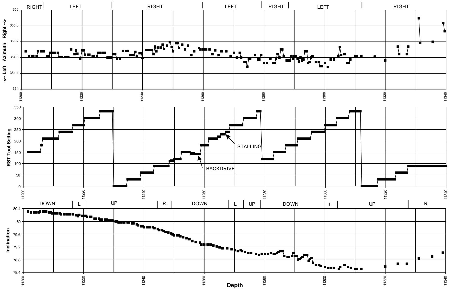
Figure 8 Auto-rotate Data Showing Wellpath Following Toolface Setting
