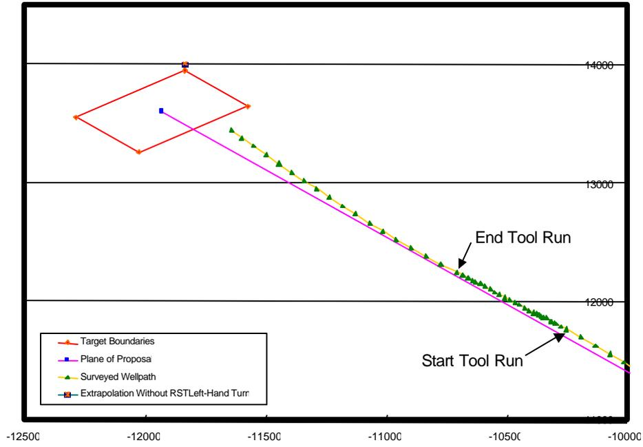
Figure 5 - Confirmation of Left Hand Turn Imparted by RST Tool
