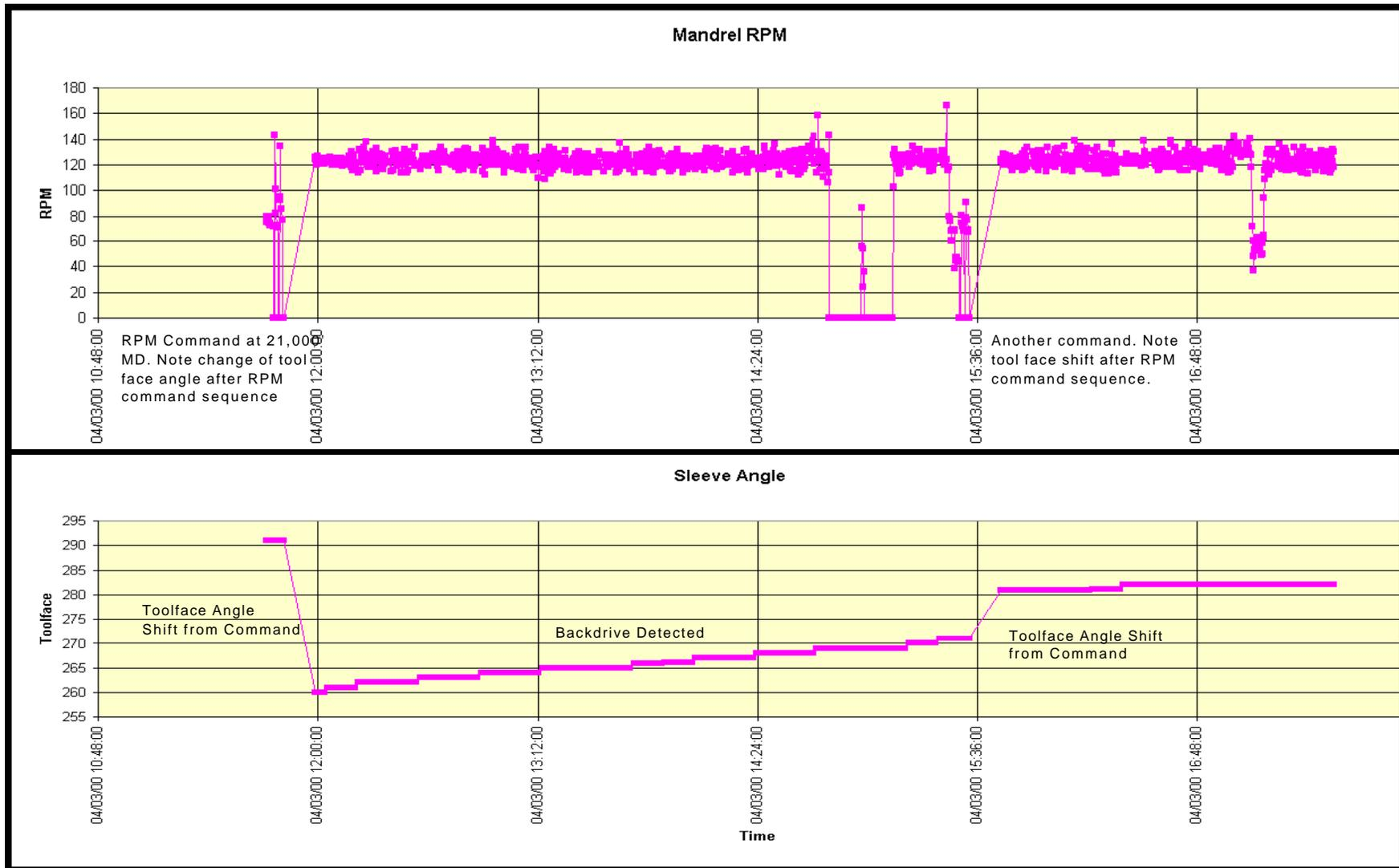
Figure 9 - Toolface Angle Shifts in Response to RPM Commands
