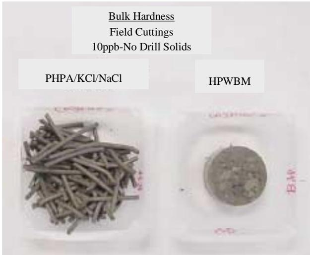
Fig 7a – Field cuttings exposed to inhibitive fluid and then extruded using the Bulk Hardness procedure.
