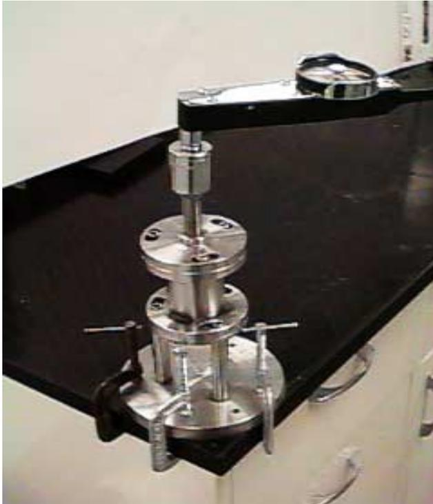
Fig 3 – Bulk hardness tester.
