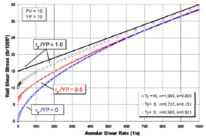
*Fig. 5: Annular flow curves comparing exact (markers) and approximate (solid lines) solutions for different R ratios (Zamora and Power 2002).*
