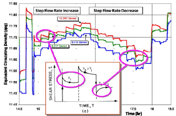
Fig. 4: Impact of flow rate step change on ECD from White *et al.* (1996) with superimposed Fig. 4.22a from Bourgoyne *et al.* (1986).
