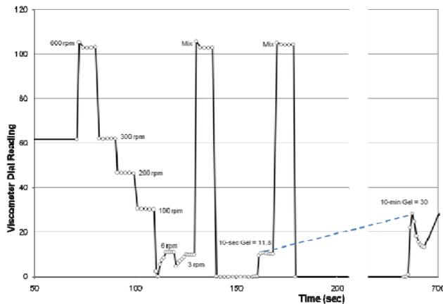
Fig. 1: Typical viscometer run. Dashed line shows gel-strength trend.
