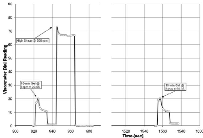
Fig. 3: Test comparing gel-strength measurements at 6 and 3 rpm showing thixotropic effects.
