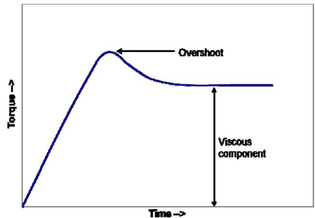
Fig. 2: Drawing showing peak and viscous components of a typical gel-strength test.
