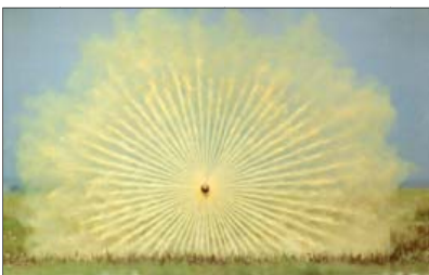
Fig. 9. Dyed water used to illustrate the radial pattern of the expelled fluid through the nozzles of a chemical cutter.
