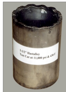
Fig. 8. Example of a Radial Cutting Torch Cut, from MCR Oil Tools.
