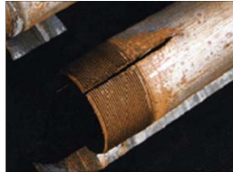
Fig. 13. Split Shot tool in 3 1/2 in. tubing, from Owen Oil Tools LP a subsidiary of Core Laboratories.
