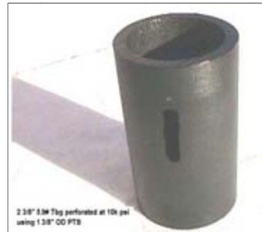
Fig. 6. Example of a non-explosive perforating torch system, from MCR Oil Tools.
