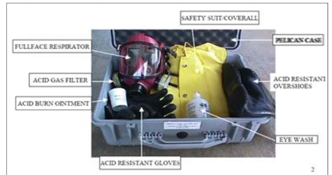
Fig. 10. Special personal protection equipment is required for chemical cutter operations.
