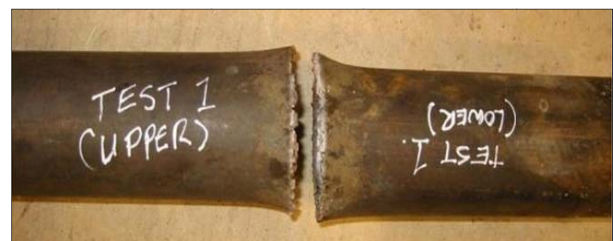
Fig. 7. A jet cut showing the flaring of the pipe.
