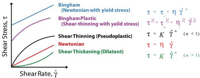
Figure 1. Fluid behavior models as a function of shear stress and shear rate (left) and equations governing models of fluidic behavior (right).
