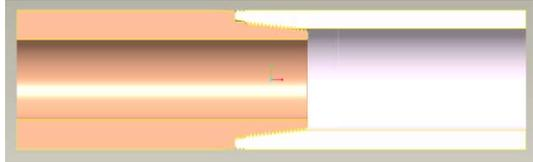
**Figure 1: Rotary Shouldered Connection (Half-section view)**
