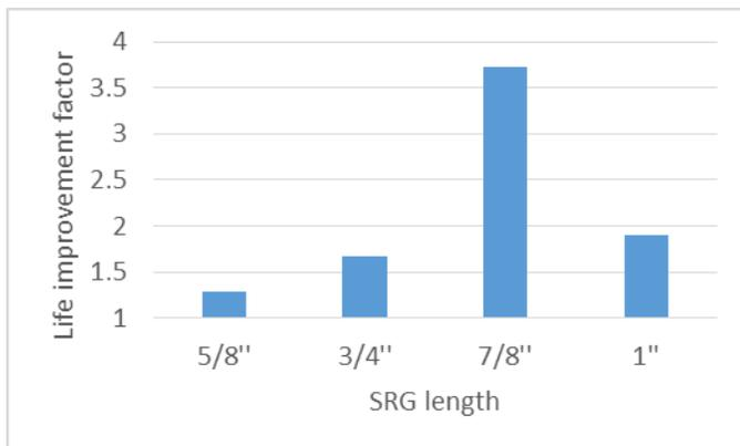
Figure 5: Fatigue life improvement of the designs with an SRG over the No SRG design as a function of SRG length.
