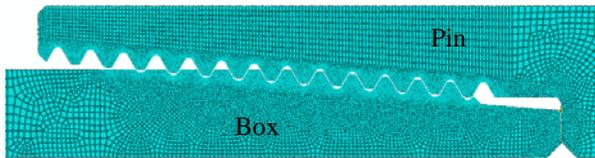
**Figure 2: Example mesh of a threaded connection.**
