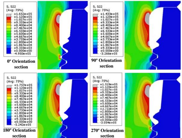
**Figure 3: Stress plots of NC38 with different sectional orientations.**
