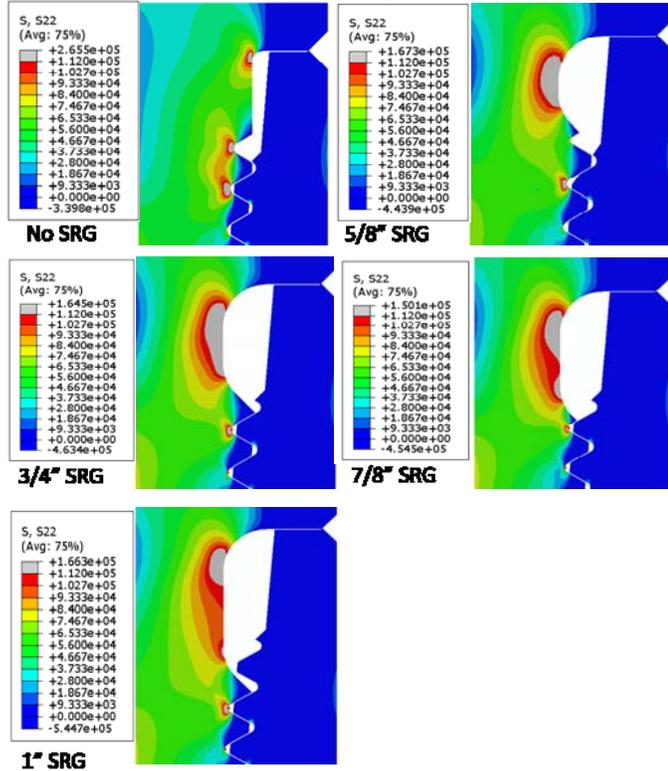
Figure 4: Stress plots of NC38 with different SRG lengths.
