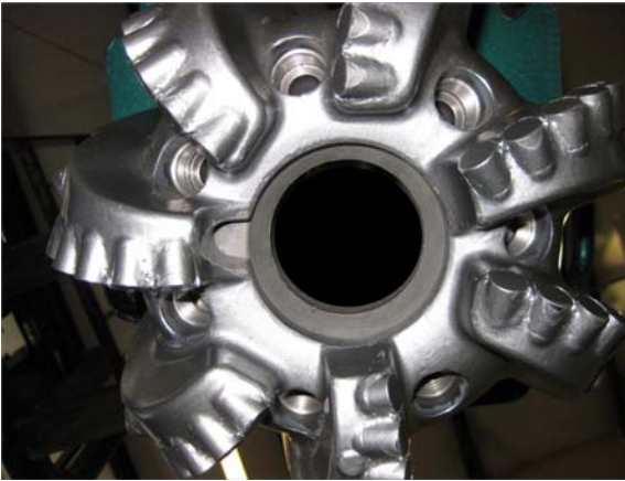
Figure 3 – The PDC through bore bit. The slim 2-1/8" tool string can easily pass through the middle in both directions.
