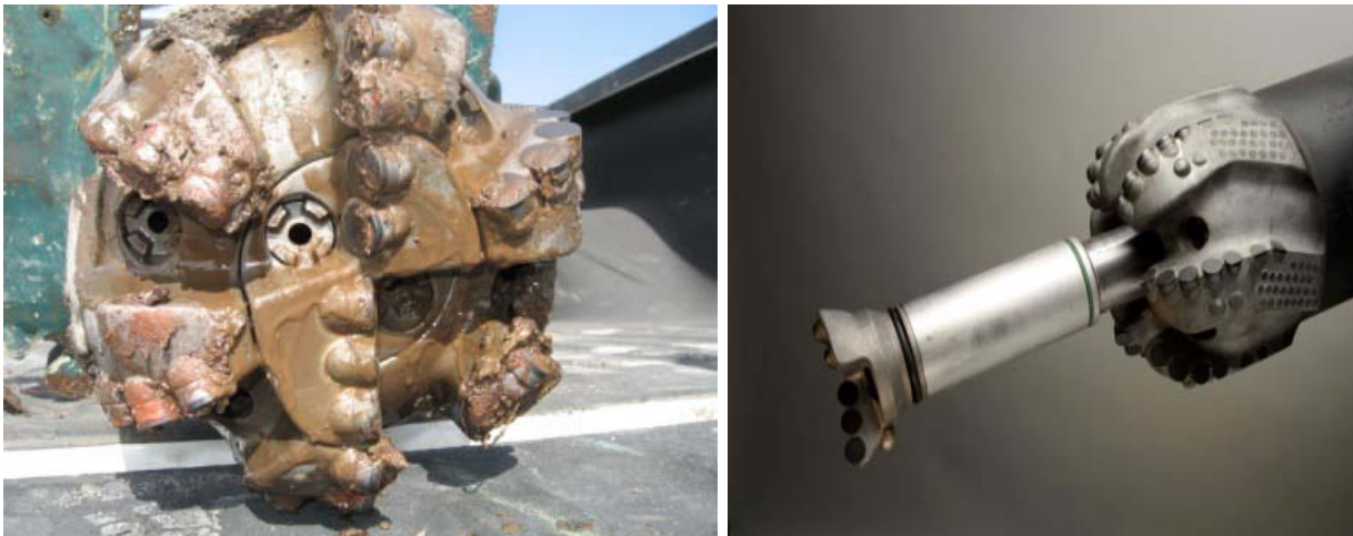
Figure 7 – A 7-7/8" through-bore bit with the center insert in place after completing a drilling run (left), and the same bit after the running tool has removed the insert and extended it beyond the bit(right). The 2-1/8" logging string is then exposed to open hole to obtain logs in either real time or in memory. After logging, the tools are retrieved and the center insert is securely reattached into the bit.
