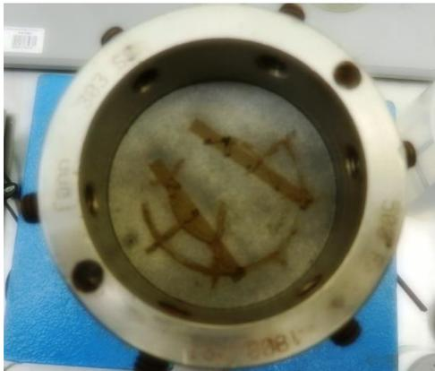
Figure 12 – Static filtration in fractured porous media – Pill D
