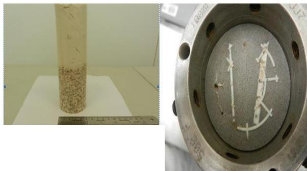
**Figure 4 – Static filtration in fractured porous media – Fluid A**
