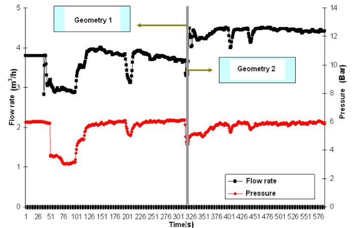
Figure 13 – Pressure and Flow rate profile at the Fracture Flow Simulator tests – Pill D
