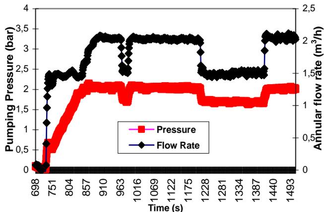
Figure 8 – Pumping pressure and annular flow rate x time – Geometry 1
