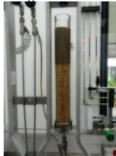
Figure 1 – Static filtration an unconsolidated bed
