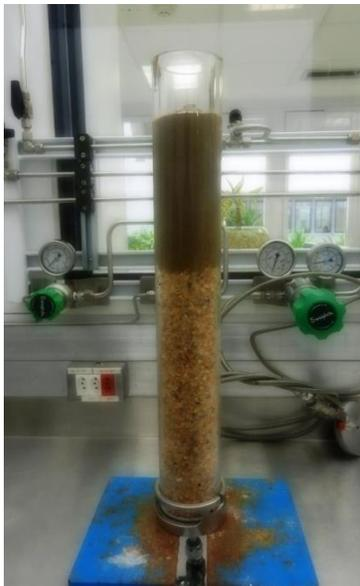
Figure 11 – Static filtration test on limestone bed – Pill D
