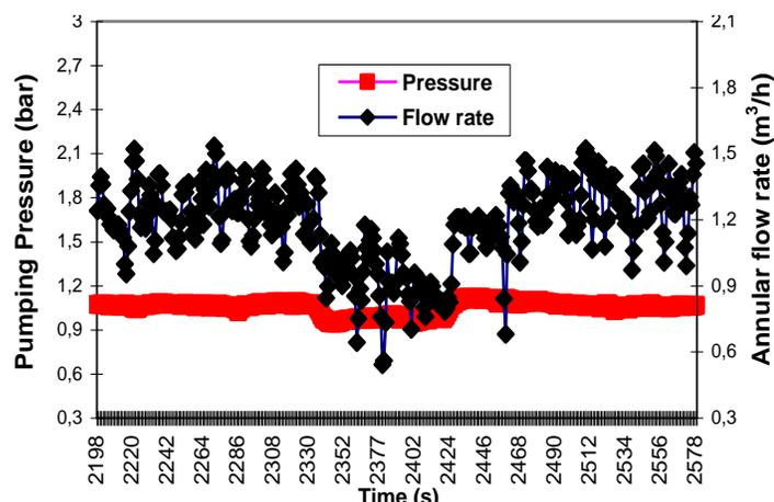
Figure 9 – Pumping pressure and Flow rate x time – Geometry 1
