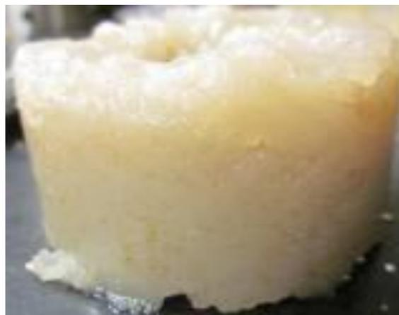
Figure 10 – Filter cake generated by Pill C1
