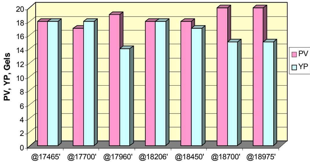
Fig. 3 - Rheology of biopolymer-free field mud measured at 120°F during the drilling operation.
