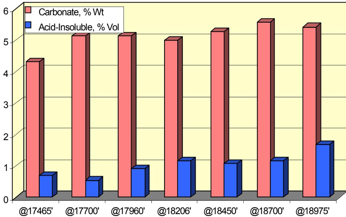
**Fig. 7 - Variation of the content of calcium carbonate and acid-insoluble materials in field mud samples. The gradual increase in calcium carbonate was related to the use of carbonate-based pills. The increase in acid-insoluble was related to the incorporation of drill solids from shale.**
