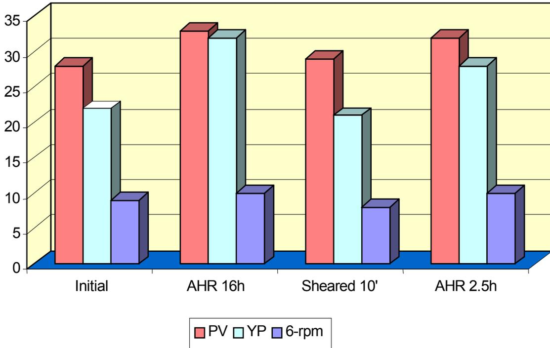
Fig. 1 – Effects of temperature and shearing on rheology of biopolymer-free drill-in fluid.
