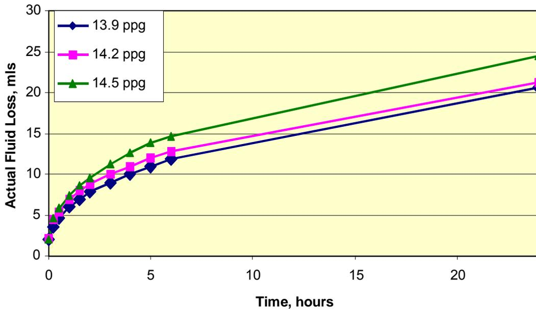
Fig. 2 – 24-hr fluid losses of biopolymer-free drill-in fluids with differing amounts of calcium carbonate as bridging material and weighting agent.
