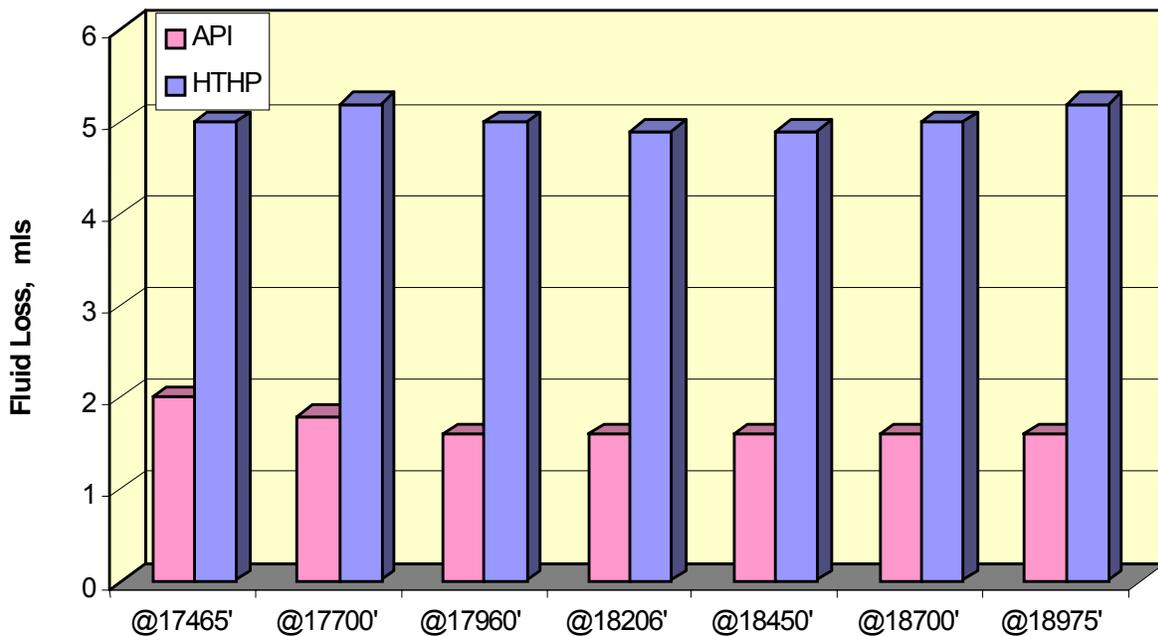
Fig. 6 - Fluid loss properties of a biopolymer-free drill-in fluid from the field trial. The fluid loss was measured at 150°F with 500 psi differential pressure over water-saturated 5-micron disk for 1 hour.
