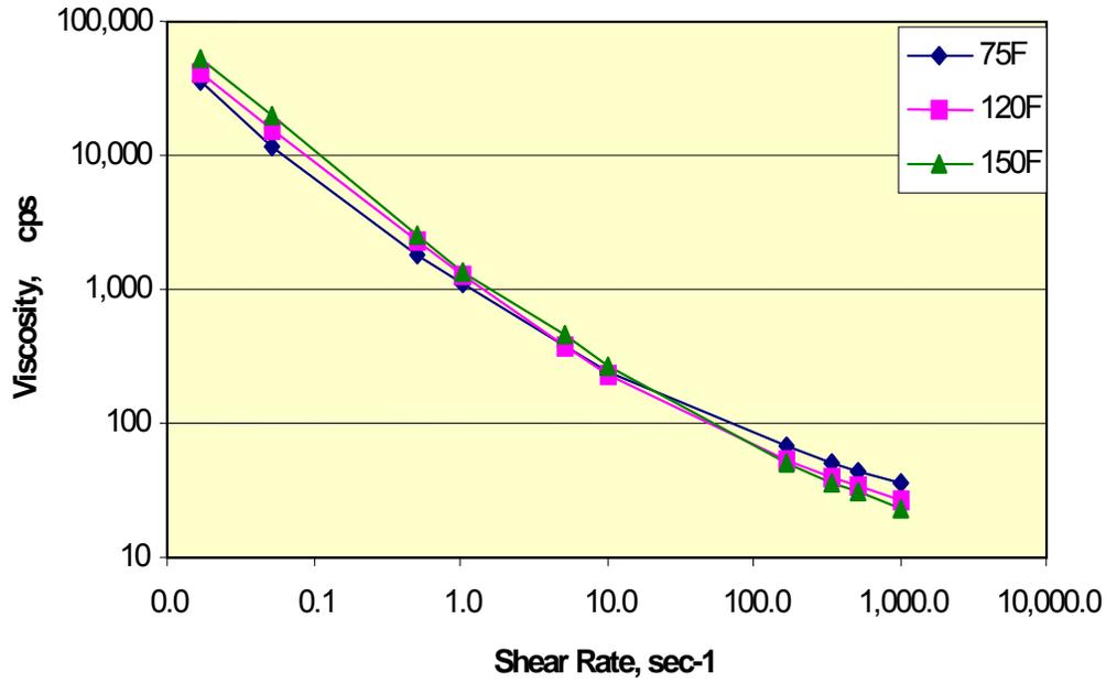
Fig 5 - A typical example of the rheological profile of the biopolymer-free drill-in fluid showing an increase of LSRV at elevated temperatures. The mud sample was collected from 17,960 ft.
