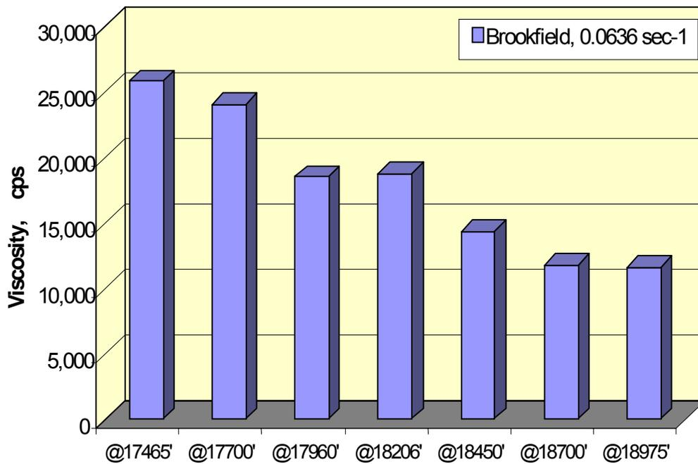
Fig 4 - Low-shear rate viscosity (LSRV) measured during the field trial of the biopolymer-free drill-in fluid. Notice the gradual decrease in LSRV with drilling. Shearing through the bit was believed to have contributed to the decrease.
