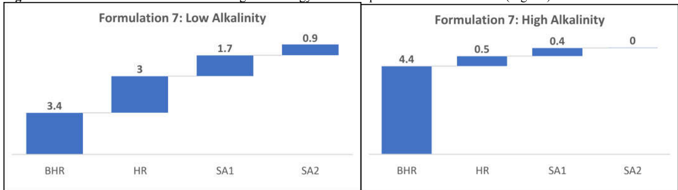
Fig. 21 —Formulation 7 showed changes in Pom (measured); the alkalinity reduced to 0 on the high alkalinity sample. A similar behavior was seen in Formulation 3 (Fig. 15).
