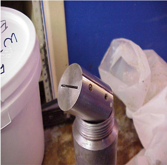
**Figure 1.** Extrusion rheometer core
