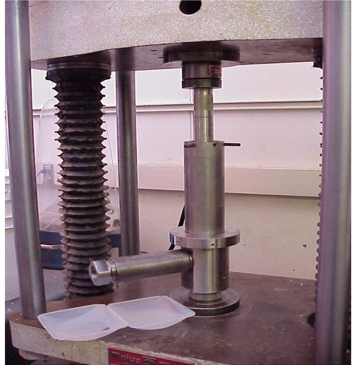
**Figure 2.** Extrusion rheometer
