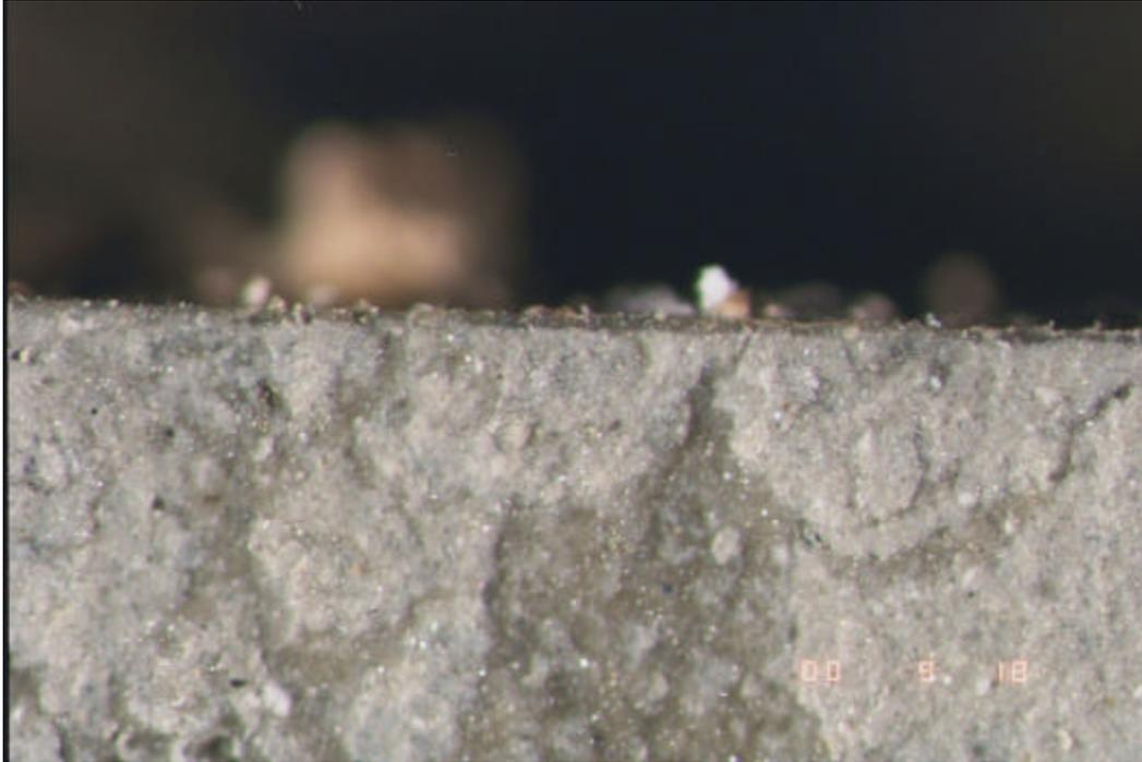
**Fig 9** Thin filtrate invasion into narrow crack.
