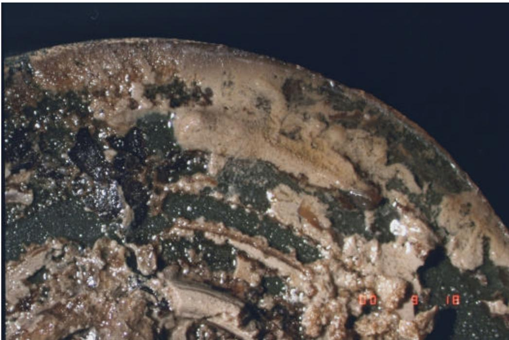
**Fig. 6** Core face with another view sealing polymer & resin complex.
