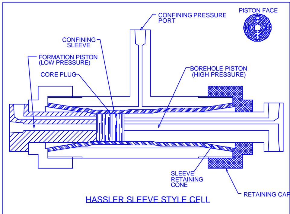
Fig. 2 Schematic diagram of pore pressure transmission apparatus.
