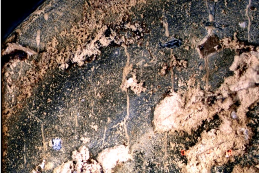
**Fig. 5** Core face with sealing polymer and resin complex.
