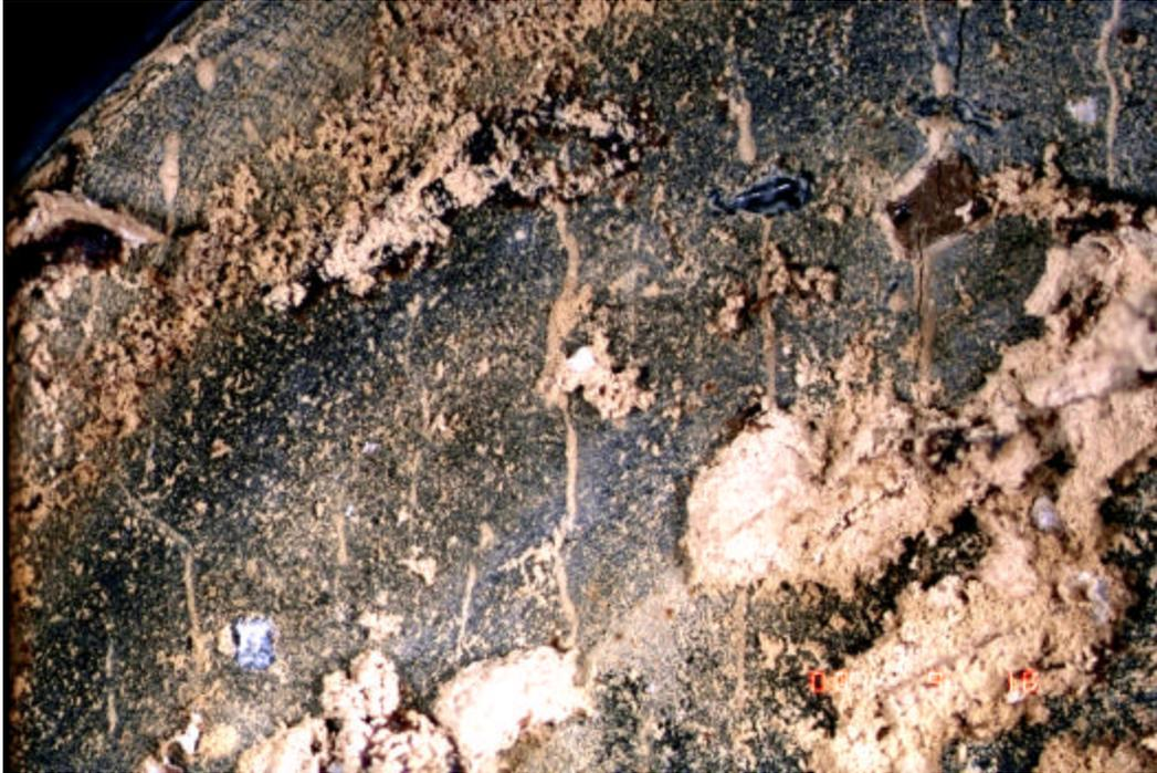
**Fig. 7** Sealing polymer covering crack.
