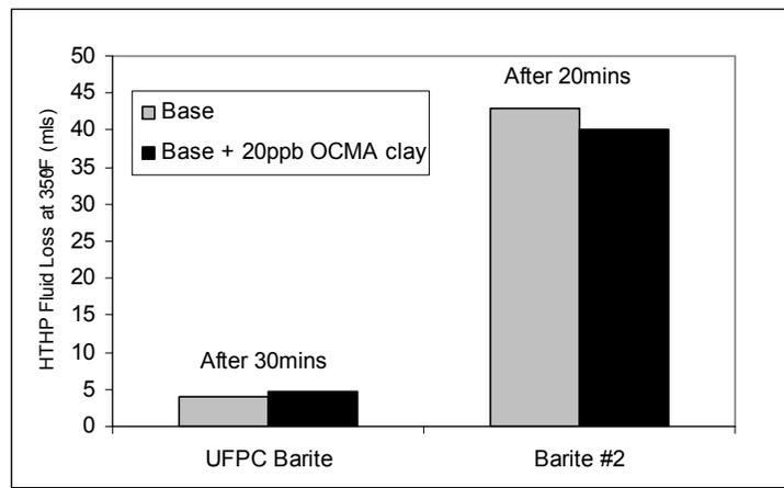
Figure 3 – Comparing HTHP Fluid Loss at 350°F
