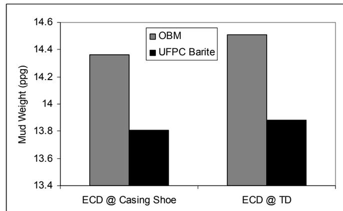
**Figure 6 – Calculated ECD's at a Flow Rate of 1800 L/min**
