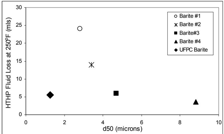
Figure 2 – Comparing HTHP Fluid Loss at 250°F
