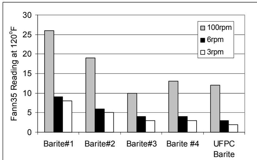
**Figure 5 – Low Shear Rheology of 14-lb/gal fluids**
