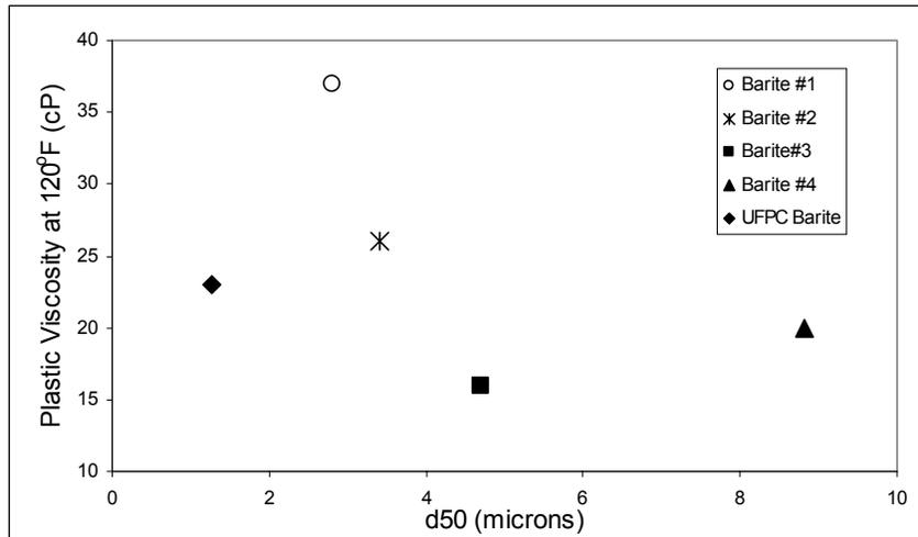
**Figure 4 – The Effect of Particle Size on Plastic Viscosity**
