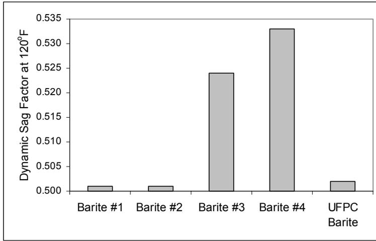
Figure 7 – Dynamic Sag after 30 min at 100-rpm at 120°F
