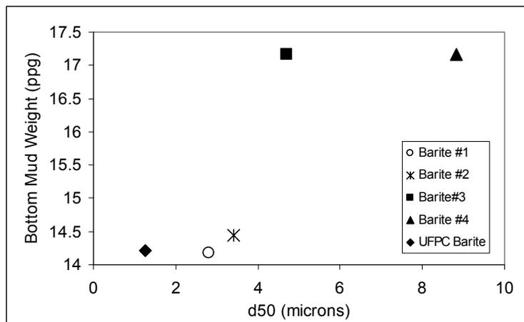
Figure 9 – Static Sag after 40 hours at 250°F
