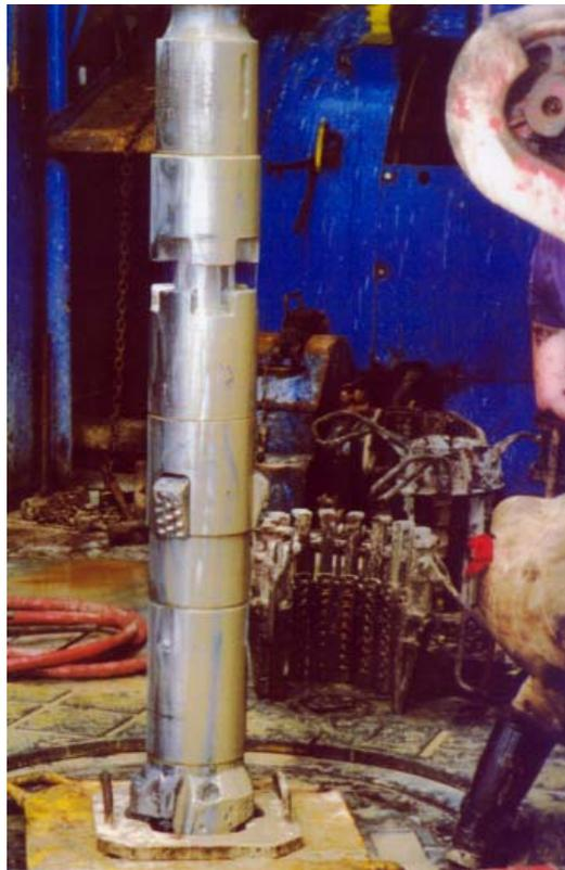
**Figure (1) – Enlarge While Drilling (EWD) Tool**
