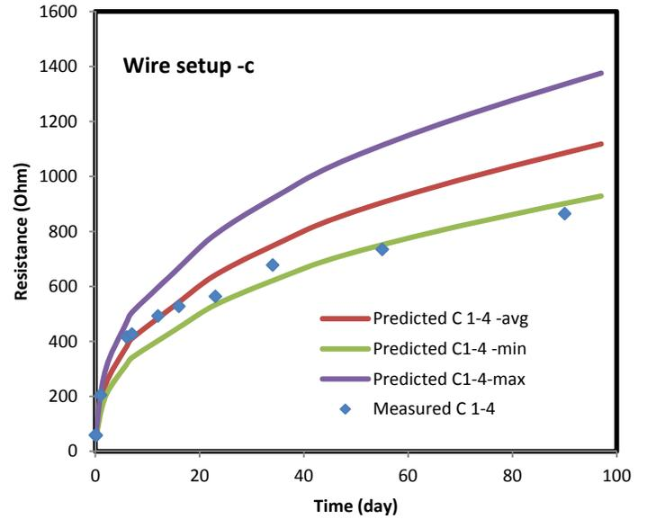
Figure 19. Predicted and measured resistance for wire setup C for wire combination c1 and c4.
