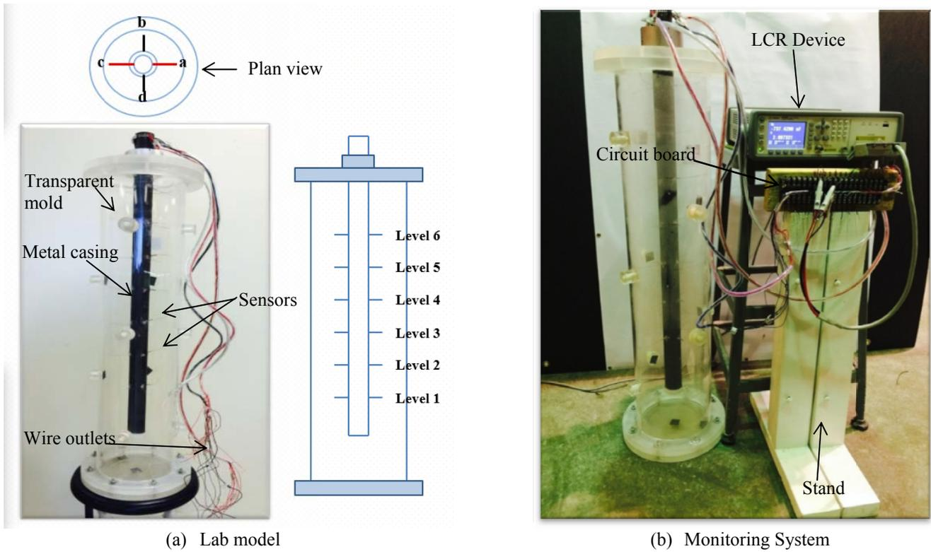
Figure 5. Laboratory scale oil well model and monitoring system
