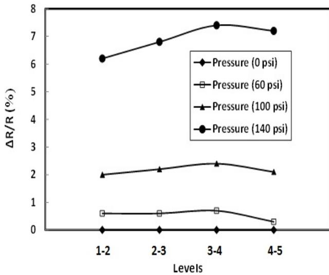
Figure 22. The changes in resistance with applied pressure for smart cement after 100 days of curing
