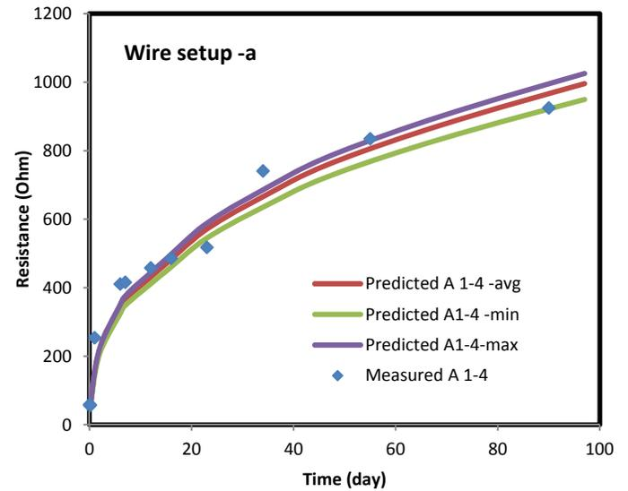
Figure 15. Predicted and measured resistance for wire setup A for wire combination a1-a4
