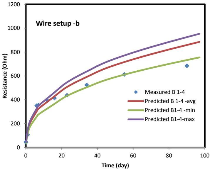
Figure 17. Predicted and measured resistance for wire setup B for wire combination b1 and b4.
