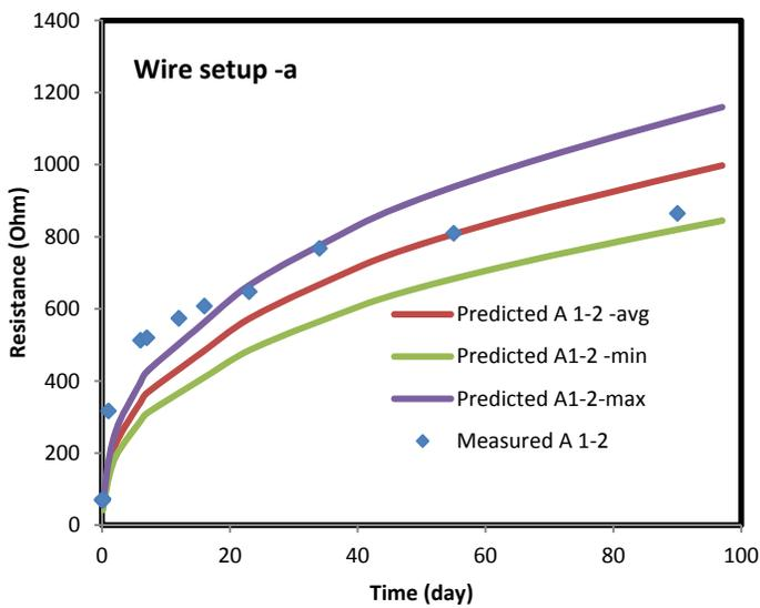
Figure 14. Comparing the predicted and measured resistance for wire setup-a for wire combination a1-a2.
