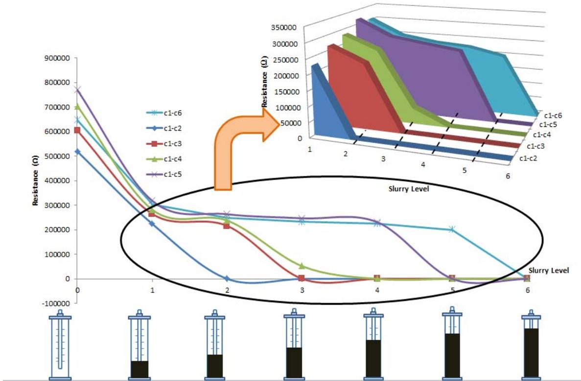
Figure 9. Variation of vertical resistance with different level of cement slurry
