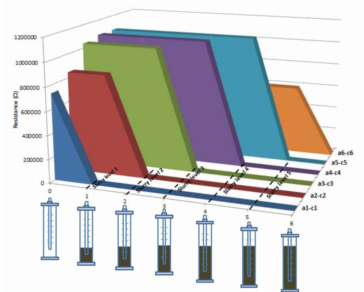
Figure 11. Horizontal slurry resistance with slurry level
