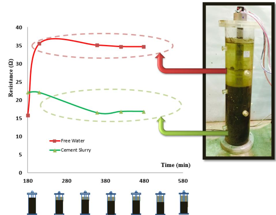
Figure 10. Resistance for free water and cement slurry
