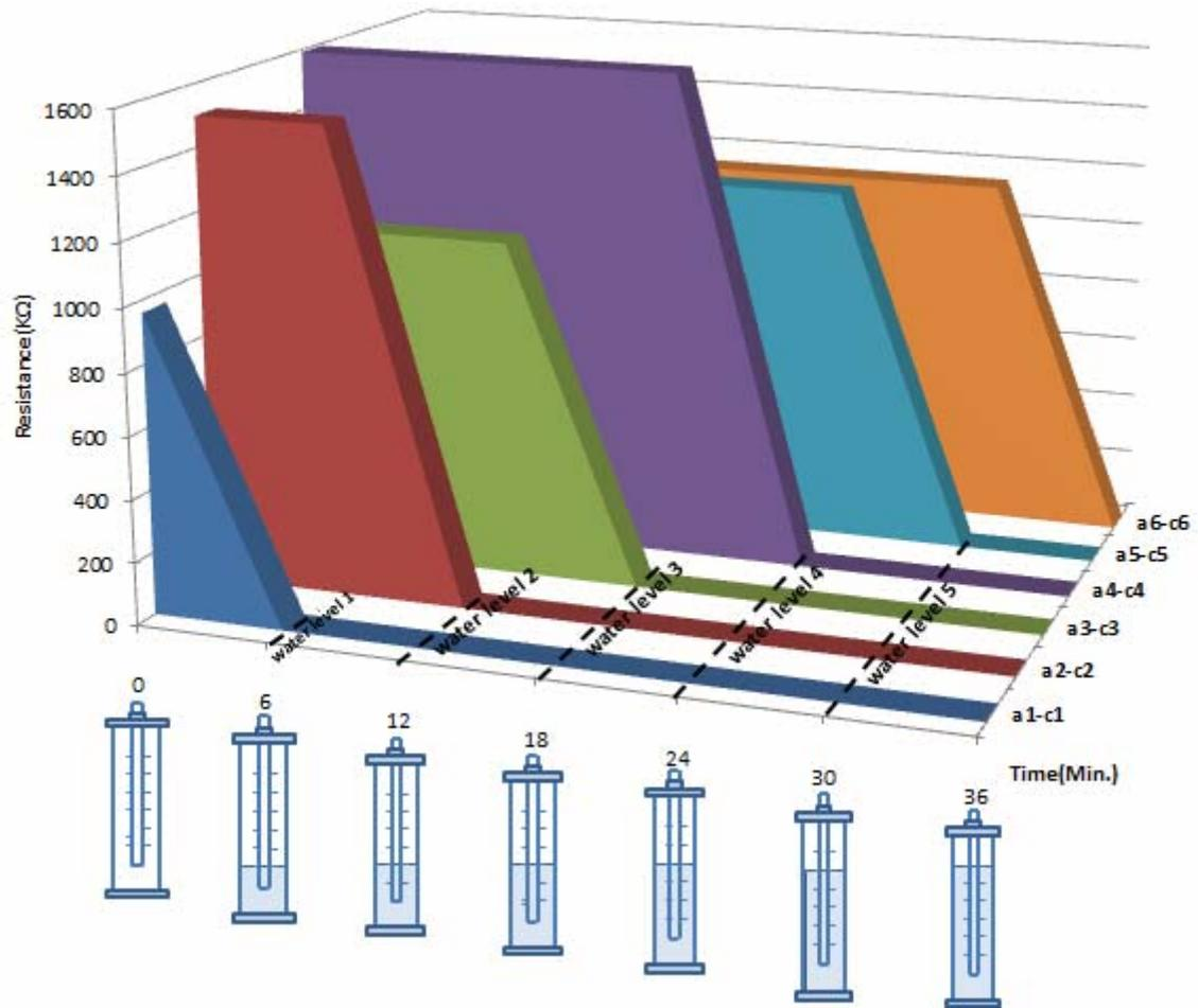
Figure 7. Horizontal resistance measurements with varying heights of water level
