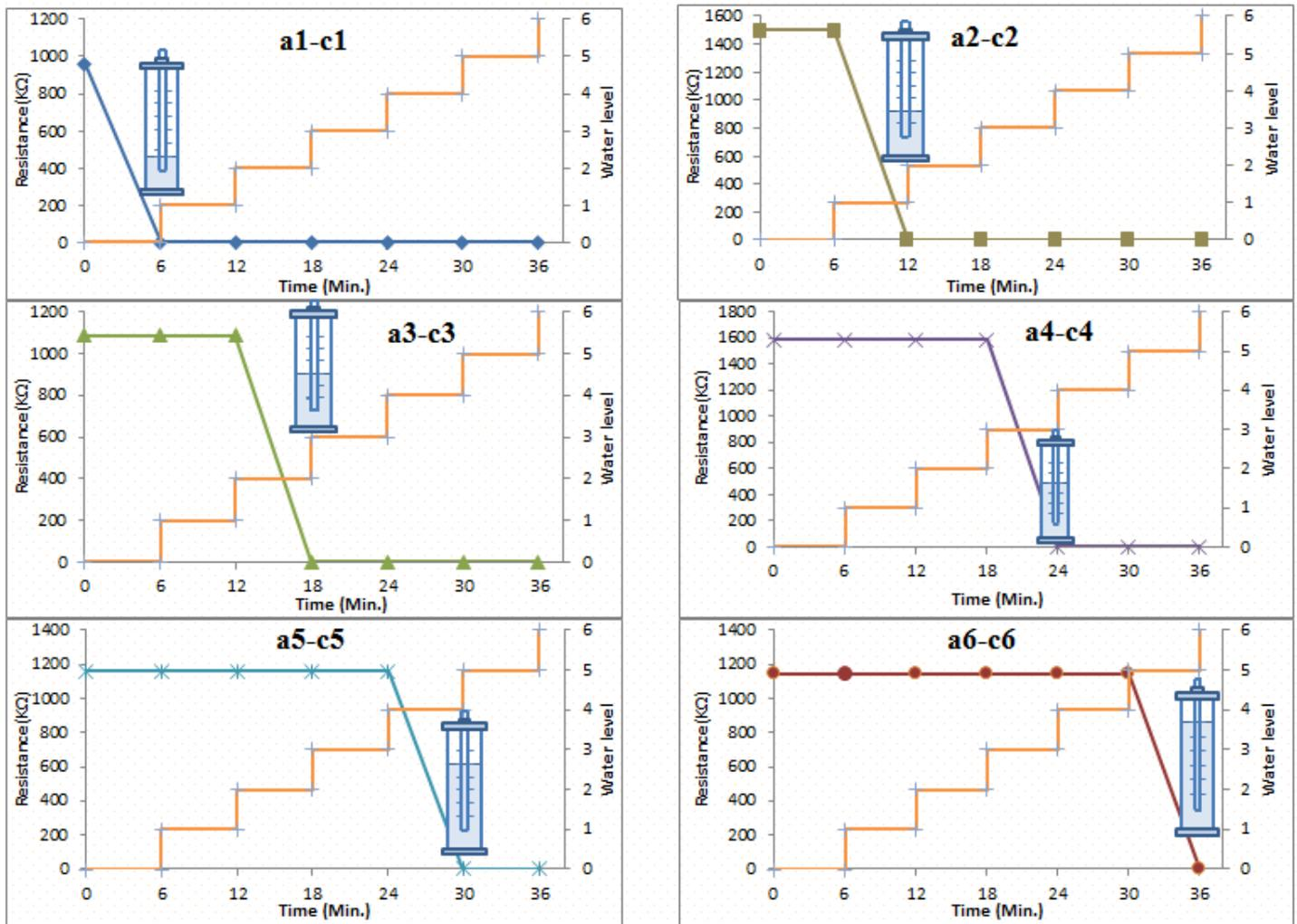
Figure 8. Variation of resistance with rising water level
