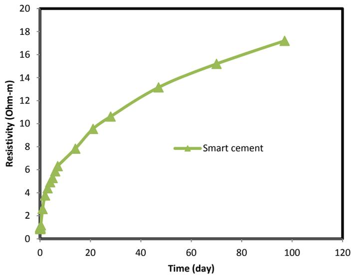
Figure 13. Variation of smart cement resistivity with curing time for samples cured under room conditions (23°C and 50% relative humidity (RH))
