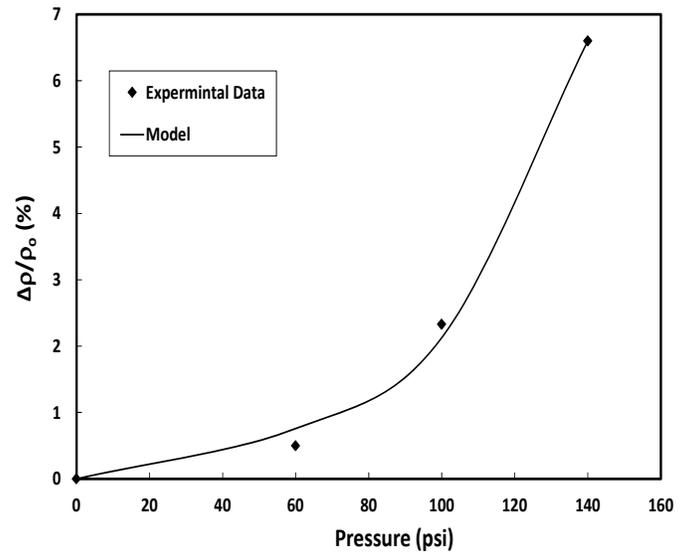
Figure 23. Model prediction of changes in resistivity with applied pressure for smart cement after 100 days of curing.
