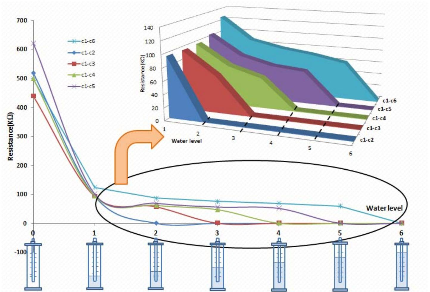
Figure 6. Vertical resistance measurement in the oil small model with changing water level
