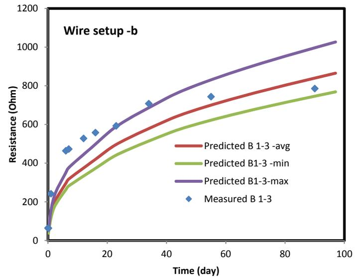
Figure 16. Predicted and measured resistance for wire setup B for wire combination b1 and b3
