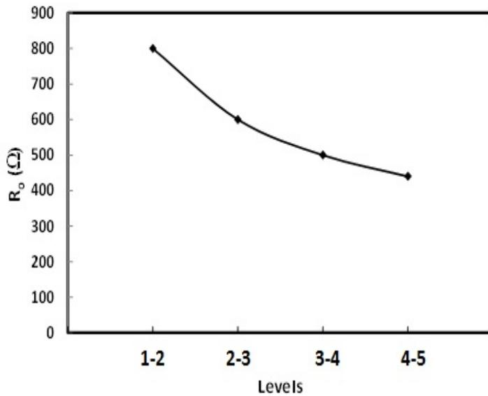
Figure 21. Variation of initial resistance with depth after 100 days of curing
