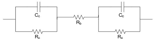
Figure 2. Equivalent circuit for Case 2
