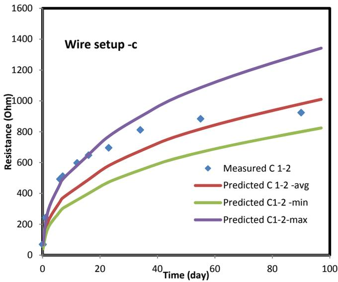
Figure 18. Predicted and measured resistance for wire setup C for wire combination c1 and c2.
