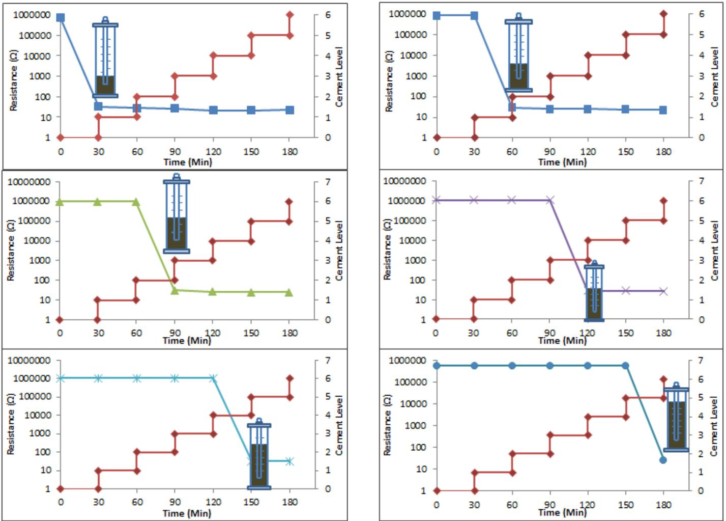
Figure 12. Horizontal resistance variation of cement slurry with slurry level
