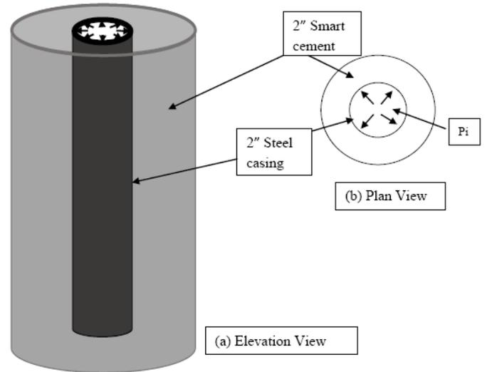
Figure 20. The configuration of the pressure applied in the inside the steel casing
