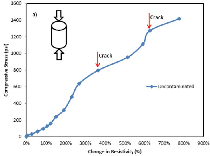
Figure 4. Typical Piezoresistivity Behavior of Oil Well Cement with 0.075% CF after one day of curing (AC frequency =300 kHz)
