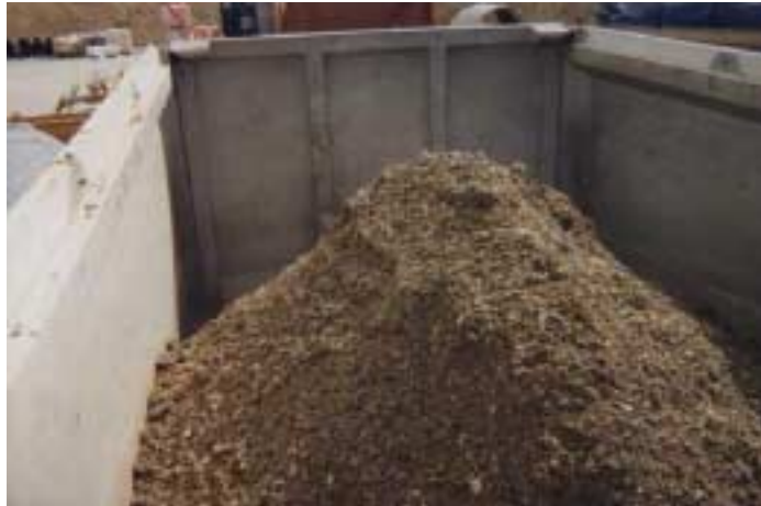
Fig. 1b - The drill cuttings mixed with sawdust ready for transportation.
