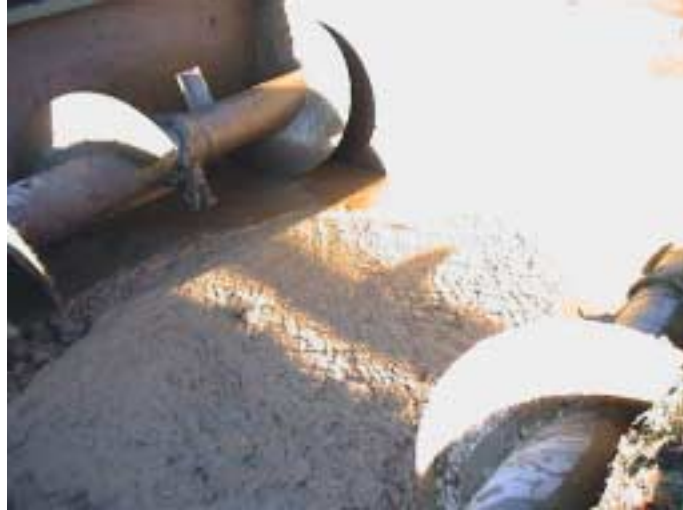
Fig. 2b - Mixing the cuttings, organic buffer and water in the feed-out wagon.
