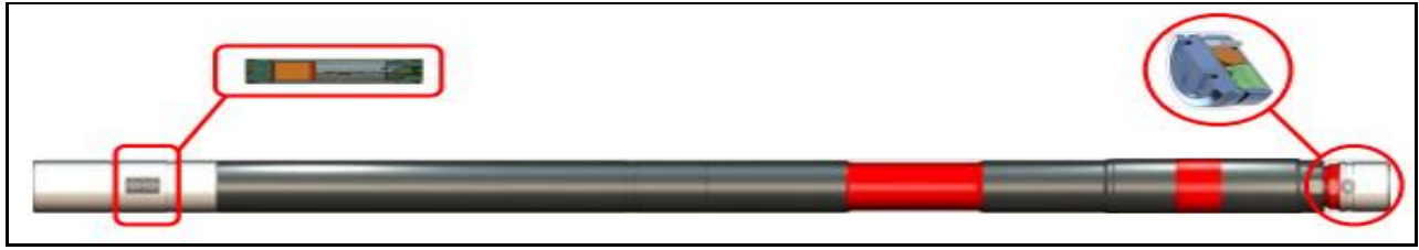
Figure 1: Mud Motor with Embedded Sensors in Bit Box and Top Sub
