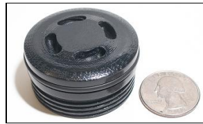
Figure 3: At-Bit Sensor Installed in a “Puck” Shaped Package
