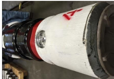
Figure 2: Sensor Installed in Motor Bit Box
