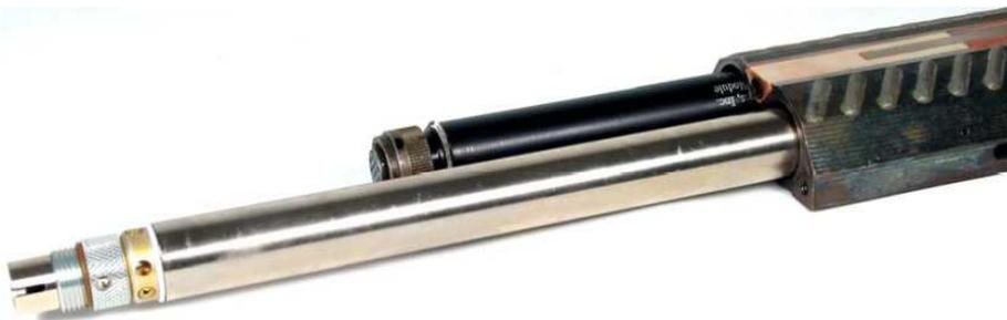
Figure 2: Instrumented motor payload showing telemetry module, sensor module and antenna
