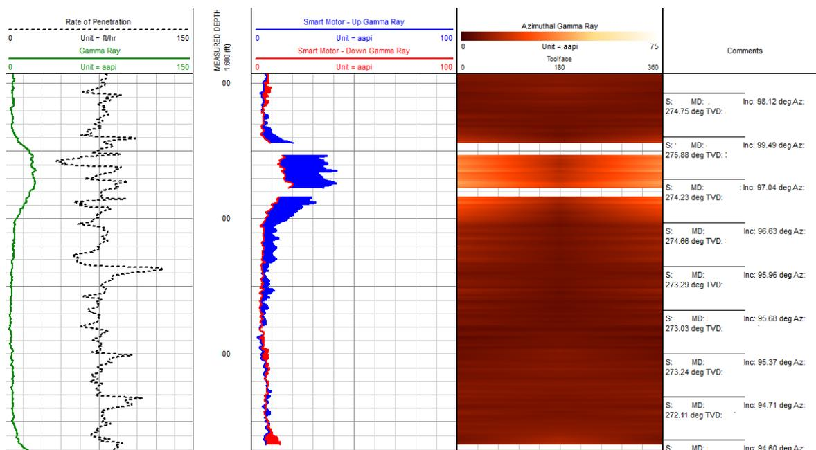
Figure 6: Log Showing Azimuthal Gamma and Inclination measurements
