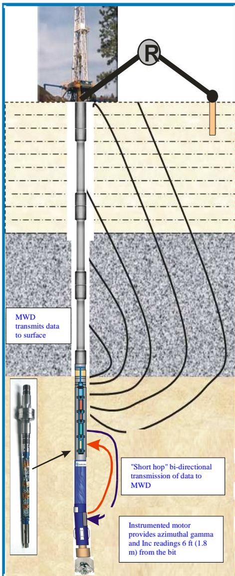
Figure 1: Near-bit Instrumented Motor with wireless bi-directional "short hop" communication and MWD system
