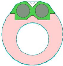
Figure 3: Cross section of instrumented motor showing payload (green)- with motor body acting as gamma shield.
