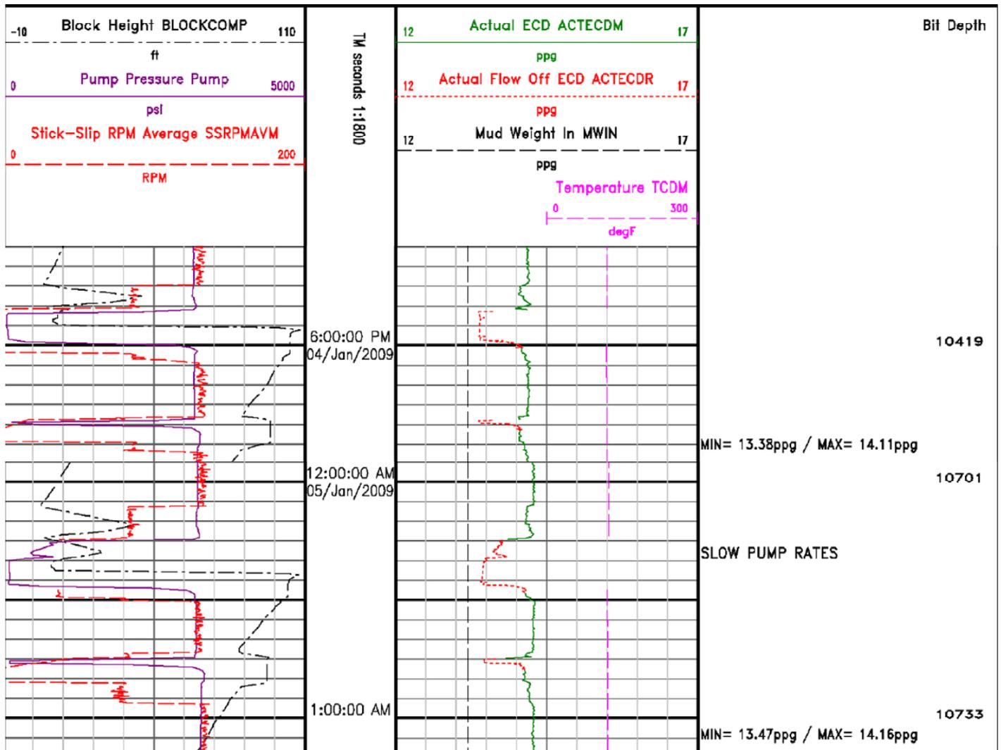
Figure 3 PWD log obtained from Well 2 (clay-free SBM) shows minimal pressure increases after static periods.
