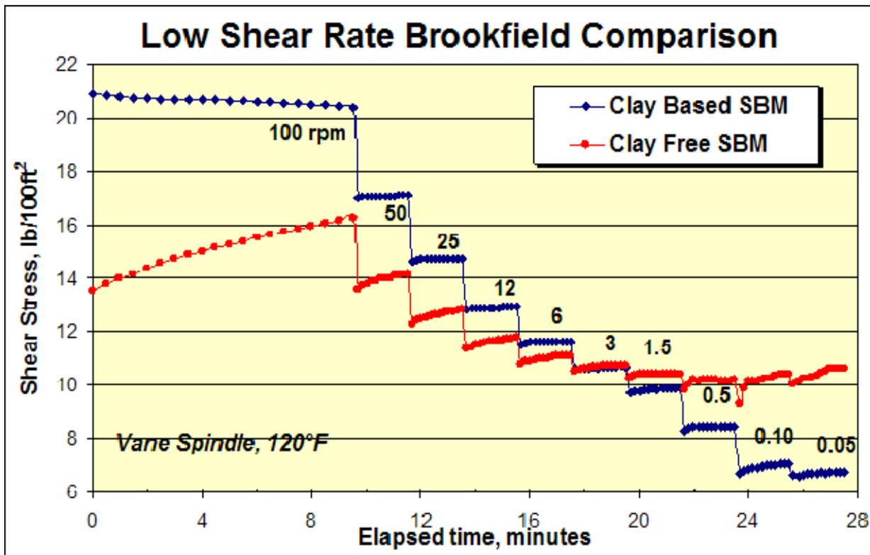
Figure 5 Comparison of ultra low shear readings for clay-based and clay-free SBMs of similar weights.
