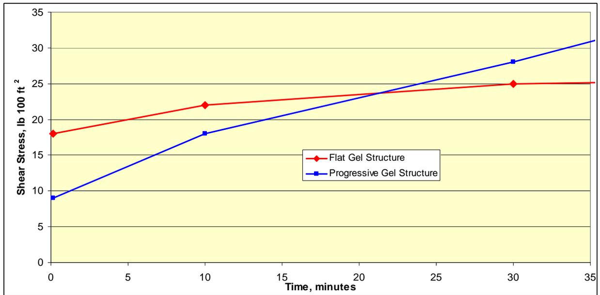
Figure 1 Gel strength development over time: flat gel vs. progressive gel.
