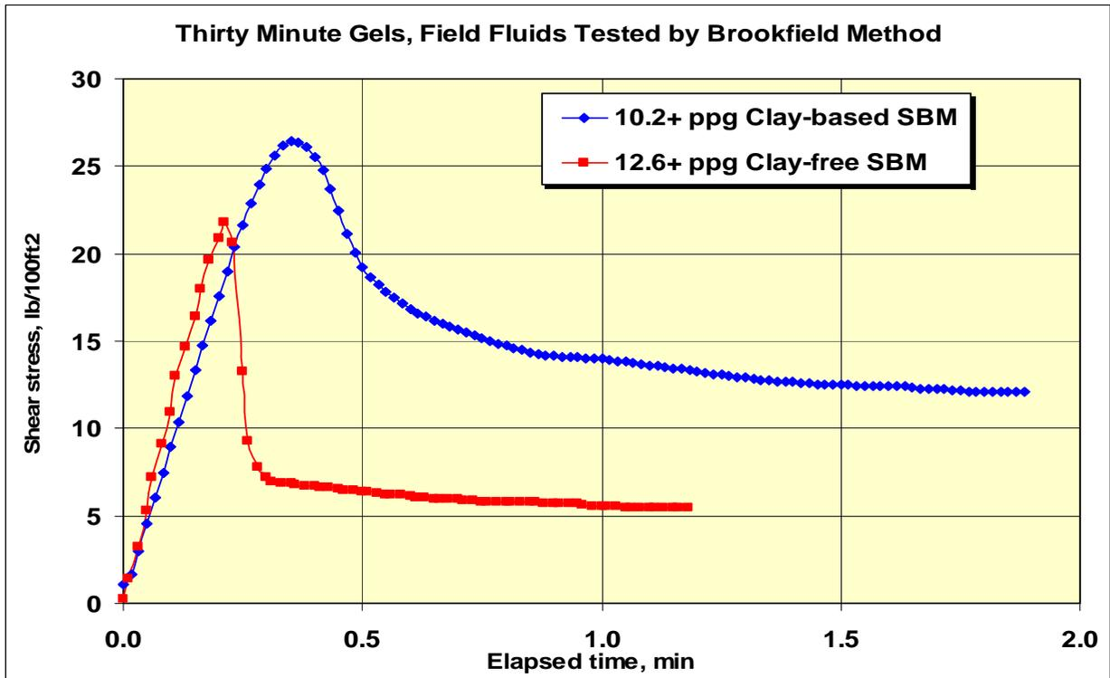
Figure 4 Comparison of shear stress required to break gel strengths built by clay-based and clay-free SBMs.
