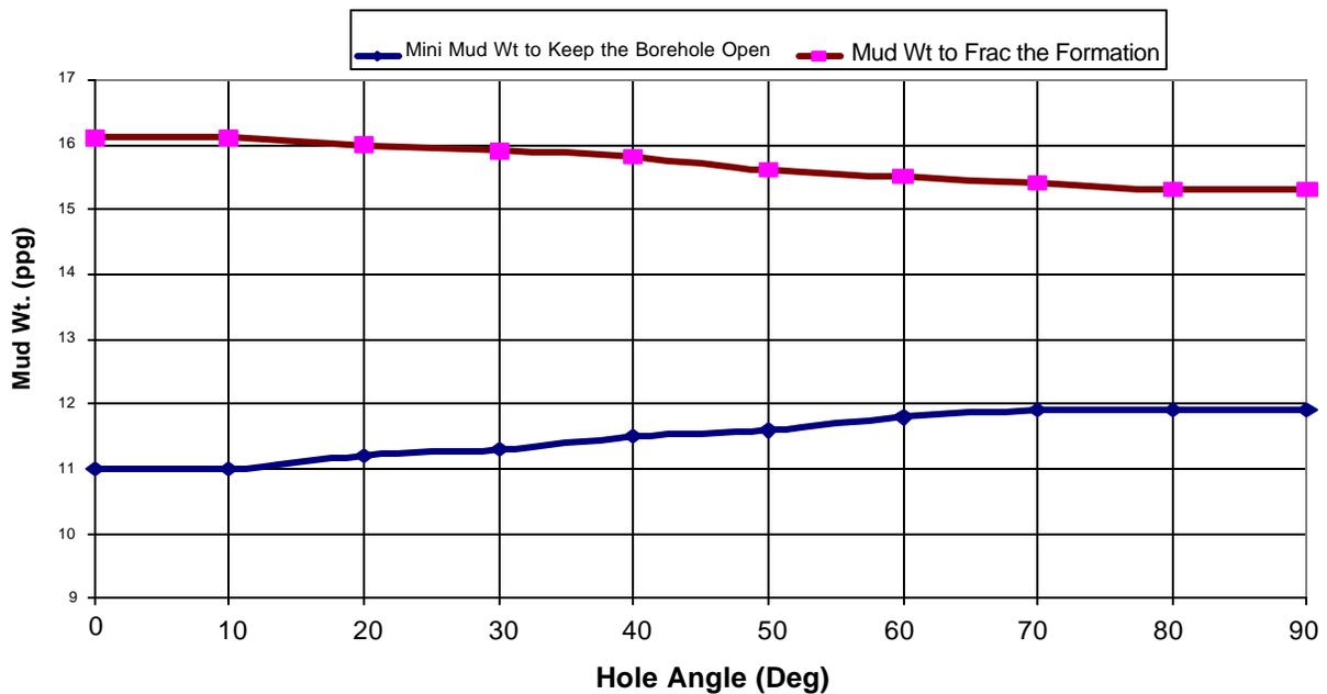
Figure 2. Example output from a linear-elastic borehole stability model showing the minimum and maximum mud weight predictions.
