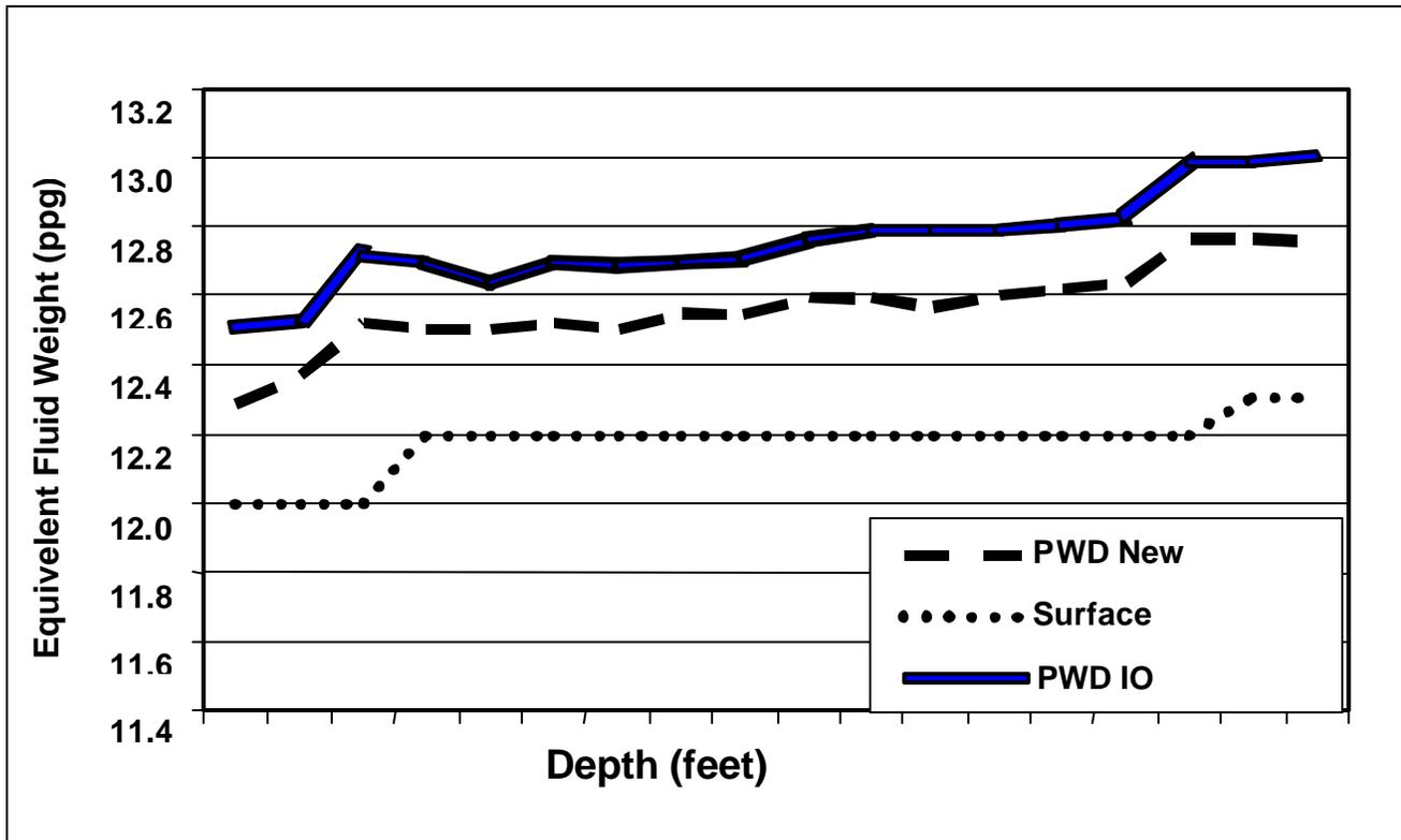
Figure 1 The New System: ECD Comparison
