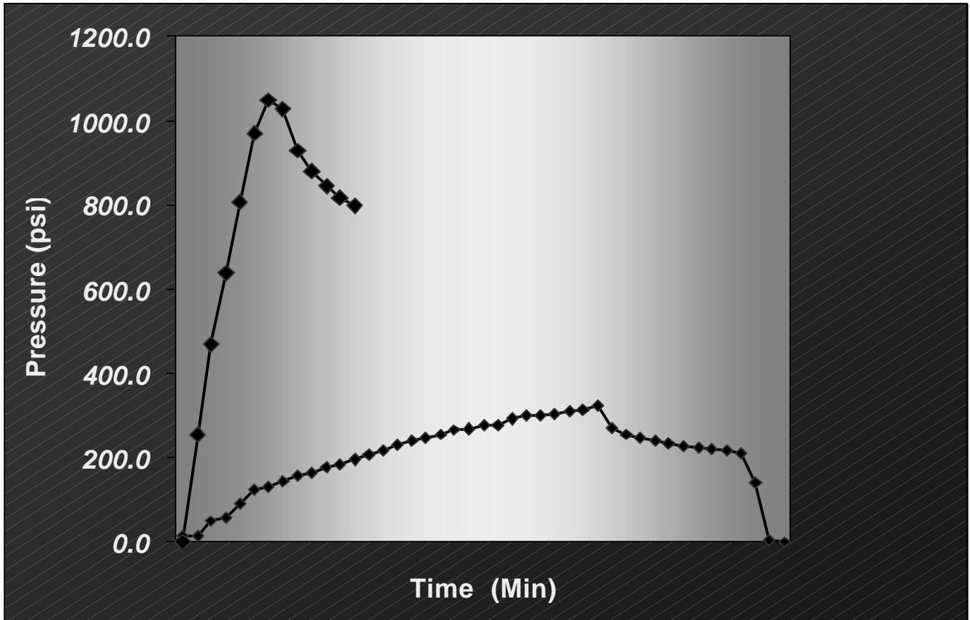
Figure 3. The before (lower curve) and after(upper curve) treatment LOT results for a deep HPHT well drilled with SBM
