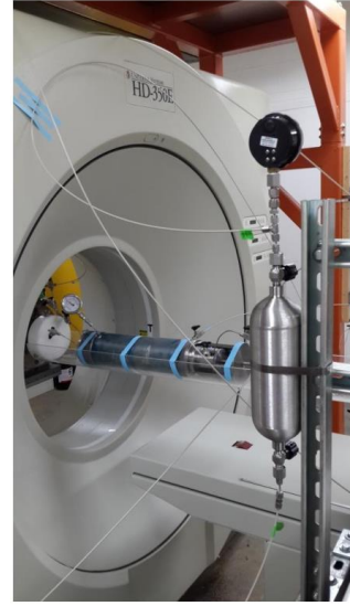
Fig. 1. Coreflood experiment conducted inside the CT scanner [13].
