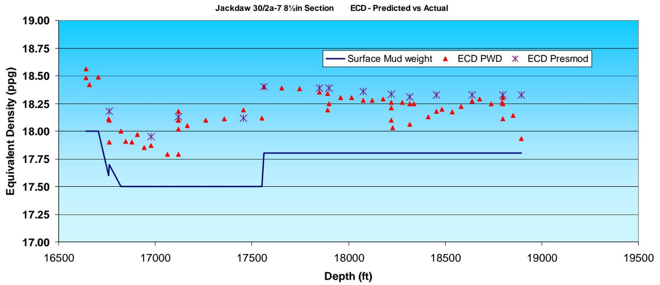
Figure 8: Comparison of measured and calculated ECD values
