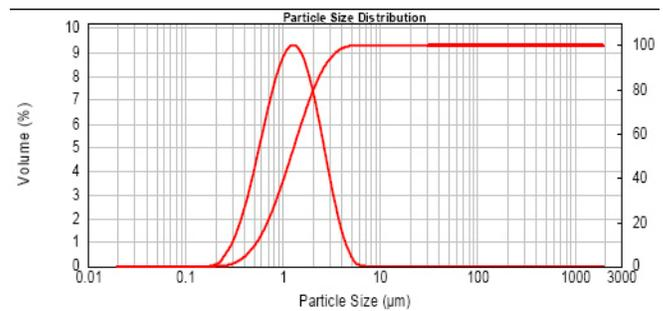
Figure 2: Manganese tetraoxide particle size distribution
