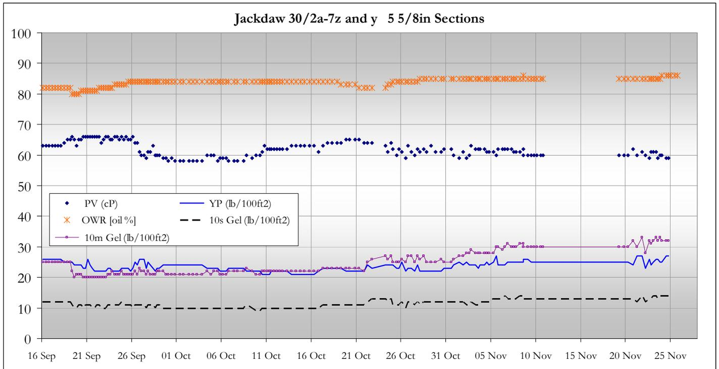
Figure 7: Mud properties as a function of time during sidetrack drilling
