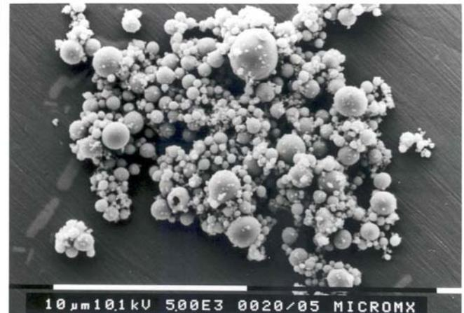
Figure 3: SEM photograph of manganese tetraoxide
