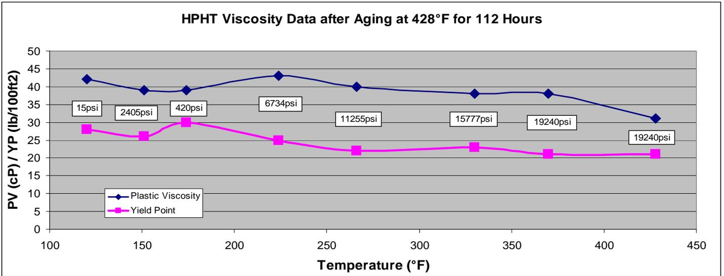
Figure 6: HPHT viscosity data for mud formulation shown in Table 3 after aging at 428°F for 112 hours
