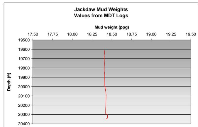
Figure 5: Hydrostatic well profile from MDT log
