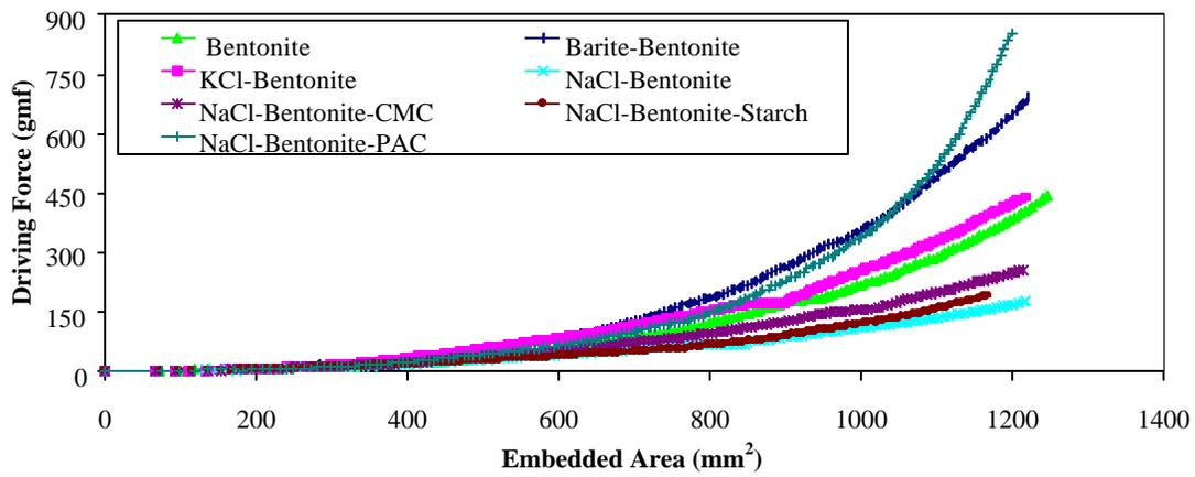
Figure13 Driving Force versus Embedded Area Curves of Different Mudcakes
