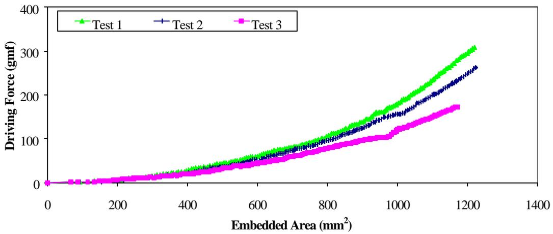
Figure 10 Driving Force versus Embedded Area (NaCl-Bentonite-CMC Mudcake)
