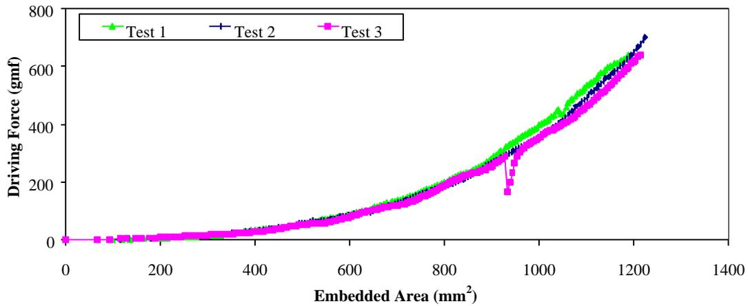
Figure 7 Driving Force versus Embedded Area (Barite-Bentonite Mudcake)
