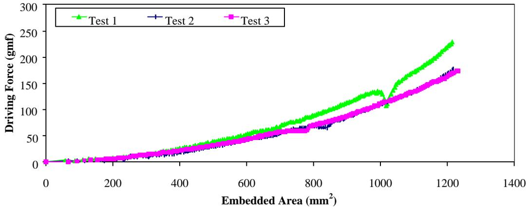
Figure 9 Driving Force versus Embedded Area (NaCl-Bentonite Mudcake)
