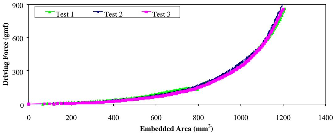
Figure 11 Driving Force versus Embedded Area (NaCl-Bentonite-PAC Mudcake)
