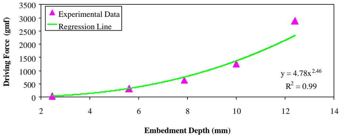
Figure 4 Driving Force versus Embedment Depth
