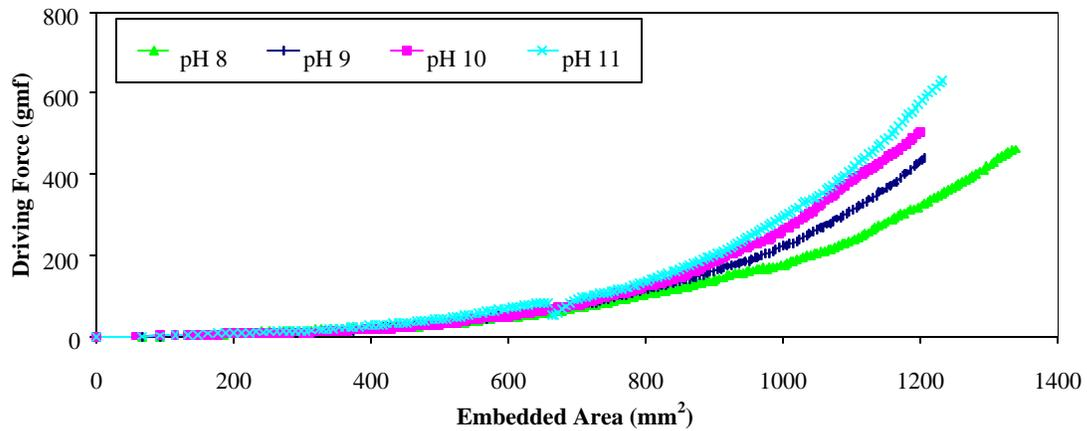
Figure 5 Driving Force versus Embedded Area for Different pH values of Mud
