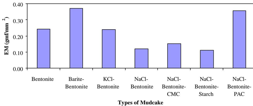
Figure14 Embedment Modulus of Different Mudcakes
