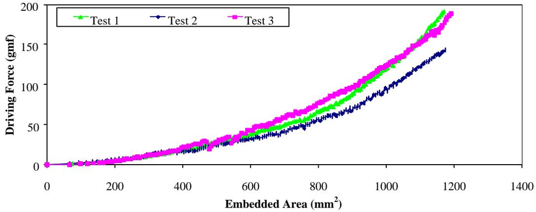
Figure 12 Driving Force versus Embedded Area (NaCl-Bentonite-Starch Mudcake)
