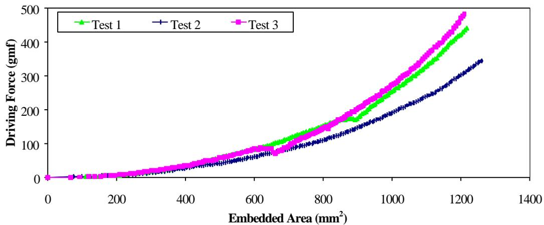
Figure 8 Driving Force versus Embedded Area (KCl-Bentonite Mudcake)
