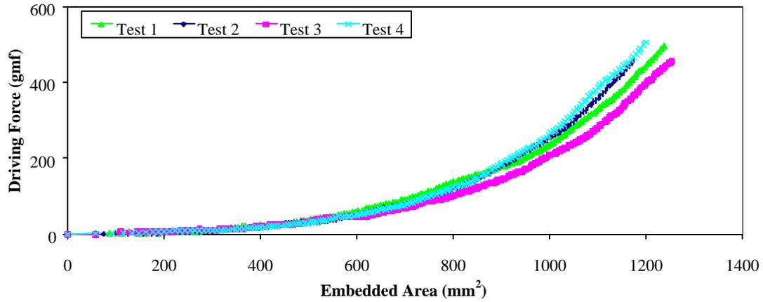
Figure 6 Driving Force versus Embedded Area (Bentonite Mudcake)
