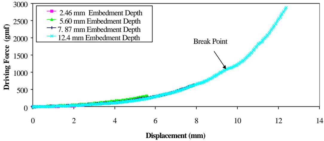
Figure 3 Driving Force versus Displacement with Different Depth of Embedment (Bentonite Mudcake)
