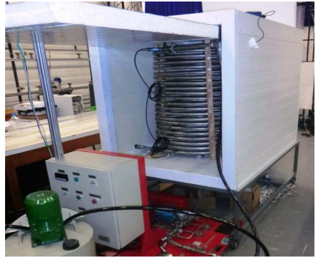
Figure 7 - Experimental rig designed for pressure transmission measurements.
